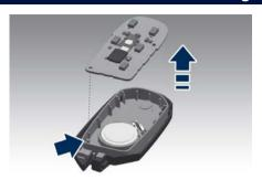
Remove the battery from its seat and replace with a new recommended type of battery.
