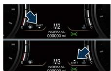
When the new gear is engaged, the GSI turns off. If the shift runs late or is not performed at all, the indicator remains lit for a few seconds then turns off. As soon as new conditions requiring further gear change occur,
