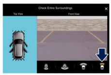
In the top view, the vehicle is represented as it is during the maneuver (see example in the figure),
