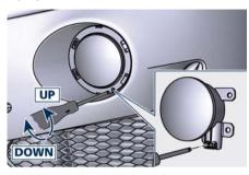
Once the adjustment is finished, remount the fog lamp frame, centering it in the seat with the longer upper and lower appendices.
