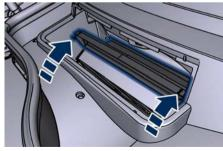
• Remove the used filter slipping it off from within the air intake.
