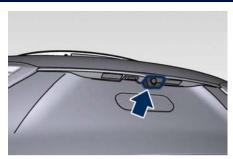
When the shift lever is shifted to R (Reverse) position, the top view and the rear view of the surrounding area will be automatically displayed on MIA display.
