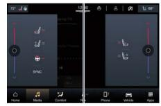
To activate and set the heating/ventilation functions of the front seats and the heating of the steering wheel (if available), in addition to what is indicated, it is possible to access the "Seats and Wheel submenu of the "Comfort" page in which there are the seats and wheel icon.
