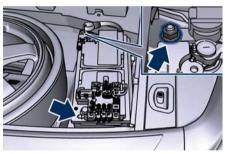
The vehicle is equipped with an IBS (Intelligent Battery Sensor) sensor able to measure charging and discharging currents and to calculate the state of charge and state of health of the battery. This sensor is located at the negative post (–) of the battery. For a successful charge/recharge operation, the charging current must
