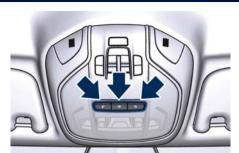
If one or more doors are opened, the front and rear dome lights will turn on for 27 seconds. If the door is closed before this time, the lights will dim and subsequently switch off after about 3 seconds.
