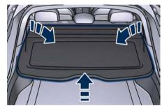
lift the cover rear end and slide it towards the liftgate: this will result in sliding the four lower ends of the cover inner part out of their guides on trunk panel;
