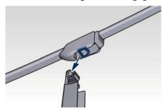
Stretch the arm and put the blade back in contact with the liftgate window.
