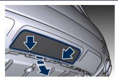
• Slide cover downward to disengage the two projecting elements indicated in the figure from bumper.
