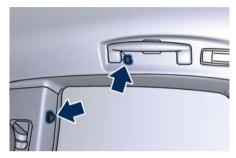
On the side walls of the trunk compartment there is a shopping hook that can withhold a maximum load of 22 lb (10 kg).
