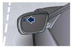
The BSA detection zone shown in figure covers approximately one lane on both sides of the vehicle (approximately 11 ft or 3.3 m). The blind spot area extends from immediately behind the exterior rear-view mirrors up to about 23 ft (7 m) behind the rear bumper.
