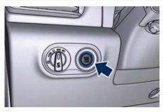
The ignition device has three operating setups indicated on the outer ring. Pressing and releasing the middle button, you can switch from one setup to the next without starting the engine, the switched on indication will turn amber.
