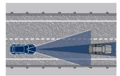
ADA combines ACC and LKA to manage the steering and speed of the vehicle under specific conditions. The conditions to engage ADA are listed in the next paragraph. If a lane line cross is imminent, the steering wheel will vibrate and a graphic will display on the instrument cluster
