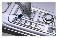
To deactivate the drive mode, press the same button again: the LED will turn off and the display will show the message indicating that \$\frac{1}{2}\$ (ESC OFF) drive mode is off and ESC system is active.
