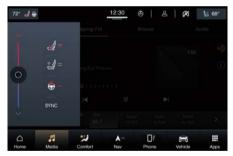
To activate the heating function, in addition to what is indicated, it is possible to access the "Seats and Wheel" submenu of the "Comfort" page in which there is the wheel icon.
