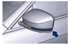
The LED turn signal indicators flash simultaneously with the corresponding turn signal lights in the front and rear of the vehicle. Turning on the hazard warning flashers will also activate these LEDs.
