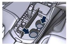
By pressing the indicated button on the central console, the half-lids will rise completely enabling access to the inner compartment where the two cupholders are located.
