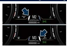
When using the transmission lever to shift, GSI indicates when a gear shift is needed by displaying just "SHIFT" on the corresponding side reinforced by an up/down arrow according to the side.
