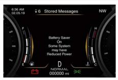
The vehicle contains advanced electronic systems, such as, for example, the alarm system and various electronic control modules, which consume power even when the ignition device is in the **OFF** position and the vehicle is not being used. Therefore, it is fundamental that the battery is properly charged to ensure that the engine starts properly and that all the electrical/electronic systems in the vehicle work efficiently.
