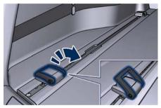
By using the Railing Fastening Bar, available in the "Genuine Accessories" range, fastened by means of sliding blocks along the floor rails, you can fasten heavy luggage in the innermost area of the trunk.
