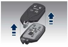
• Remove the card with PCB (Printed Circuit Board).
