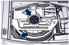
• Fit the adapter on the wrench. Extend the wrench as shown, then loosen by approximately one turn, the five bolts on the wheel to be changed. In case a wheel security stud bolt is installed, it can only be removed by using the specific fitting wrench insert provided with the "Wheel Security Stud Bolt Kit", available in the "Genuine Accessories" range. In this case, the insert must be installed on the kit wrench.
