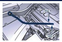
• If a refilling is necessary: unscrew the filler neck cap.
