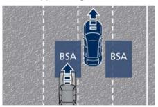
When the vehicle is started, the BSA warning light will momentarily illuminate in both outside rear view mirrors to let the driver know that the system is operational and on. The BSA system sensors operate when the vehicle is in any forward gear
