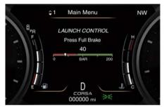
With brake pedal pressed full with left foot, fully press the accelerator pedal (with right foot) as indicated in the message on the instrument cluster.
