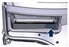
Close the filter retaining cover and reinstall the access door.
