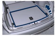
It is possible to maintain the cargo floor in the lifted position when trunk cover is not hooked to liftgate (figure 1), is hooked to liftgate (figure 2) or is removed (figure 3).
