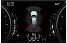
As the vehicle moves closer to the object, the instrument cluster will display the arc moving towards the vehicle and the sound tone will change from single to slow, to fast and to continuous.
