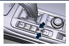
To disable the SPORT mode without activating the CORSA mode, press the same button once again: the two LED will turn off.
