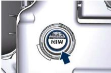
When additional engine coolant (antifreeze) is needed to maintain the proper level, it should be added to the coolant reservoir after removing the cap. Do not overfill.
