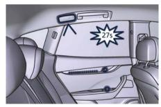
• If the lock command of the car is enabled by pressing the specific button on the key fob or by the "Passive Entry" system, when the key fob is out of range, all the lights will turn off within 3 seconds, if they were previously on.
