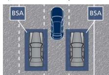
The BSA system monitors the detection zones on both sides of the vehicle
