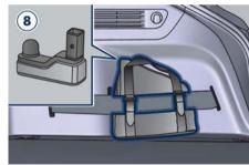
Once these operations are completed, stretch band and fasten it at the back of cargo floor, making sure to match the Velcro inserts. Lower the cargo floor.
