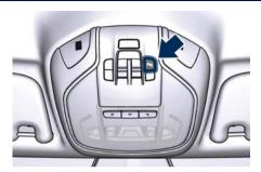
After pressing the button the instrument cluster will display the state of front parking sensors for approximately five seconds. The button LED will be on when the front sensors are disabled. The button LED will be off when the front sensors are enabled. If the button is pressed and the system requires service, the LED will blink momentarily, and then the LED will be on.
