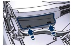
• Unsnap both ends and lift the filter retaining cover.
