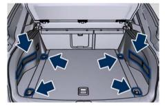
Longitudinal rails on trunk floor provide safe anchorage for luggage of different size, thanks to the special hooks with locking button. To position the hook, slide it along the rails until reaching the required position, holding down the central button. Release the button and slightly move the hook to secure its position in the notches of the guide.
