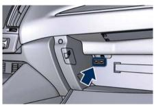
In the compartment of the central console there is also a SD memory card port. Once inserted into the slot, to extract it, press lightly on the card. For rear seat passengers, there are two USB ports inside the compartment located on the rear end of the central console, above the air vents.
