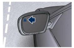
The external of the rear-view mirror support is equipped with LEDs, lighting up when the turn signals and vehicle entry/exit lights are activated.
