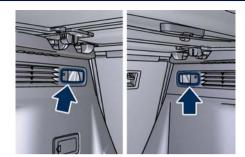
If liftgate is left open for a long time, lights will turn off after 30 minutes to save battery charge.
