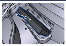
Install the new filter with arrows pointing in the direction of airflow, which is toward the rear of the vehicle (text and arrows on the filter will indicate this).
