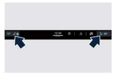
Front seats and steering wheel comfort setting soft-keys are present even when the A/C is off.
