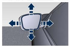
To adjust a rearview mirror, press either the L (left) or R (right) button to select the mirror that you want to adjust. The spin button will illuminate indicating the rearview mirror is activated and can be adjusted. Press the mirror control switch corresponding to the arrow indicating the direction of the desired movement.
