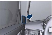
The fixed vents under the dashboard are aimed at ventilating the lower part of the front passenger compartment.
