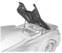
Hold until the tonneau cover is completely opened. The turn signals will flash once.
