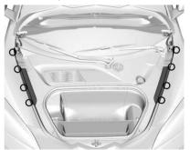
Release the four clips for the left and right outer covers.
