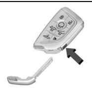
Press the button on the side of the remote key and pull the mechanical key out.
