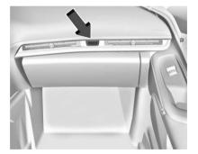
Press the button to open. Lift to close. The glove box locks when the car alarm is armed. See Vehicle Alarm System \$\simeq\$ 22.
