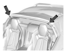
5. Position the rear edge of the roof panel next to the weatherstrip on the back of the roof opening. Then align and fit the pins at the rear of the roof panel inside the openings in the rear overhead weatherstrip. Gently lower the front edge of the roof panel to the front of the roof opening.
