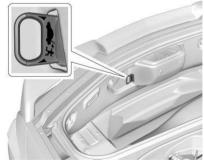
There is a glow-in-the-dark emergency hatch/ trunk release handle on the inside back wall of the storage compartment. This handle will glow following exposure to light. Pull the release handle to open the hatch/trunk from the inside.
