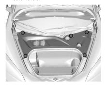
Release the five clips and remove the outer cover.
