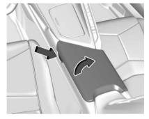
To open, press the button on the driver side. Depending on the options, there may be two USB ports inside.
