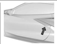
For Keyless Access, hold the remote key within 1 m (3 ft) of the door handle. Grip and press the door handle touchpad. See Remote Key Operation ▷ 8. This feature can be programmed. To view available settings from the infotainment screen, touch Settings > Vehicle > Remote Lock, Unlock, Start.
