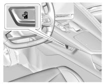
Press the Charge+ button on the driver side of the center console. When the Charge+ feature is active, the hybrid battery charging light displays on the DIC. See *Hybrid Battery Charging Light (Charge+)* ⇒ 87. Also, a small pop-up window will also appear showing the exact SOC and electric power input/output. The Hybrid Battery Gauge shows the increasing SOC filling into the blue zone. See *Power Indicator Gauge* ⇒ 87.
