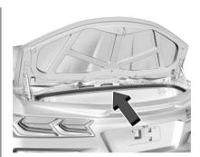
Use the pull cup to lower the hatch if needed, then drop into the latch or push on the outside of the panel until the power latch feature activates. The hatch/trunk will close the rest of the way and latch automatically.
