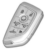
: Press to lock both doors and the fuel door. The turn signal indicators may flash and/or the horn may sound on the second press to indicate locking. To view available settings from the infotainment screen, touch Settings > Vehicle > Remote Lock, Unlock, Start.
