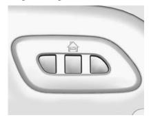
If equipped, these buttons are in the sunshade. This system can replace up to three remote control transmitters used to activate devices such as garage door openers, security systems, and home automation devices. These instructions refer to a garage door opener, but can be used for other devices.
