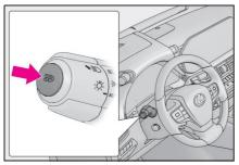
1 Press the Automatic High Beam switch.
