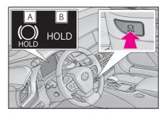
Turns the brake hold system on
