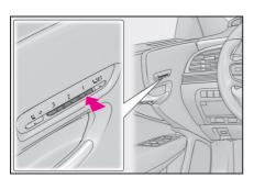
Press one of the buttons for the driving position you want to recall until the buzzer sounds.
