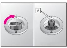
2 Turn the upper knob of each retaining hook (clip) to secure the floor mats in place.
