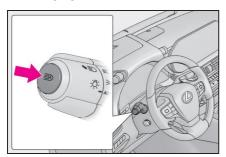
Press the Automatic High Beam switch.
