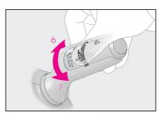
When AUTO is selected, the sensor sensitivity can be adjusted by turning the switch ring.
