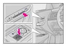
While pressing the recalled button, press and hold the door lock switch (either lock or unlock) until the buzzer sounds.
