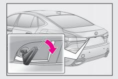
Turn the mechanical key clockwise to open.
