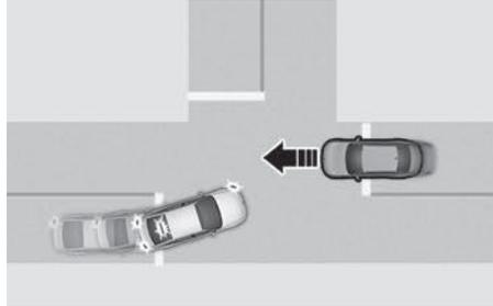
Junction Turning function can help avoid a collision with an oncoming vehicle, powered two-wheeler in an adjacent lane when turning left at a crossroad with the turn signal on by applying emergency braking.
