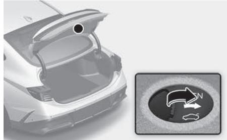
Your vehicle is equipped with the emergency trunk safety release lever located on the bottom of the trunk.
