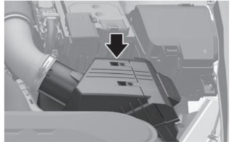
The air cleaner filter can be cleaned for inspection using compressed air.
