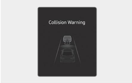
While Smart Cruise Control is operating, when the collision risk with the vehicle ahead is high, the "Collision Warning" warning message will appear on the instrument cluster with a warning sound and the steering wheel will vibrate to warn the driver. Always have your eyes on the road while driving, and if necessary, depress the brake pedal to reduce your driving speed in order to maintain a safe distance.
