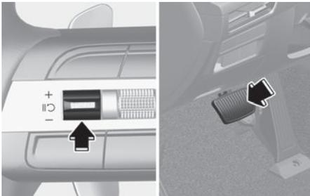
Press the (II C) switch or depress the brake pedal to temporarily cancel Smart Cruise Control.
