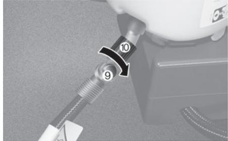
4. Connect the sealant bottle to the compressor.
