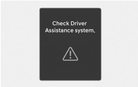
When Reverse Parking Collision-Avoidance Assist or other related functions are not working properly, the "**Check Driver Assistance system**" warning message will appear on the instrument cluster, and Reverse Parking Collision-Avoidance Assist will turn off automatically. We recommend that your vehicle be inspected by an authorized HYUNDAI dealer.
