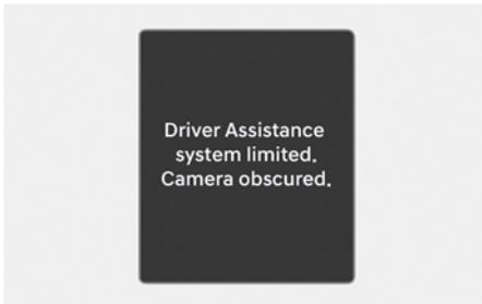
When the front windshield where the front view camera is located is covered with foreign material, such as snow or rain, it can reduce the detecting performance and temporarily limit or disable Intelligent Speed Limit Assist. If this occurs, the **"Driver Assistance system limited. Camera obscured."** warning message and the speed limit (E) warning light will appear on the instrument cluster.
