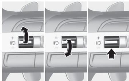
To resume Manual Speed Limit Assist after the function was paused, operate the +, -, or (LIMIT) switch.
