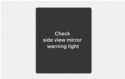
When the side view mirror warning light is not working properly, the "**Check side view mirror warning light**" warning message will appear on the instrument cluster for several seconds, and the master warning light (⚠) will appear on the instrument cluster. If this occurs, have your vehicle inspected by an authorized HYUNDAI dealer.
