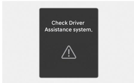
When Smart Cruise Control is not working properly, the "**Check Driver Assistance system.**" warning message and the master (⚠) warning light will appear on the instrument cluster. Have your vehicle inspected by an authorized HYUNDAI dealer.
