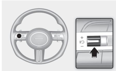
Press the (LIMIT) switch to temporarily pause the set speed limit. The set speed limit will turn off but the Speed Limit (LIMIT) indicator will stay on.
