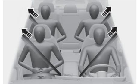
Your vehicle is equipped with driver's, front passenger's and rear passengers pretensioner seat belts (retractor pretensioner). The pretensioner makes sure the seat belts fit tightly against your body in certain frontal or side collision(s). The pretensioner seat belts may be activated in some crashes where the frontal or side collision(s) is severe enough, together with the airbags.
