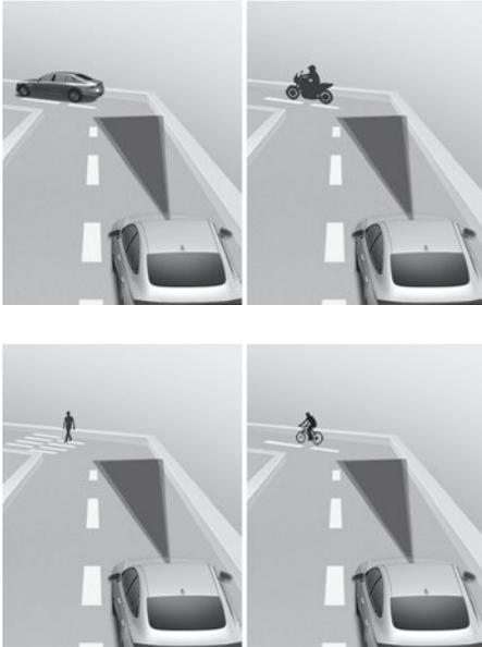
Forward Collision-Avoidance Assist may not detect a vehicle, a powered two-wheeler, a pedestrian, or a cyclist in front of you when driving on curved roads adversely affecting the performance of the sensors. This may result in no warning, braking assist when necessary.
