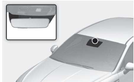
The rain sensor located on the upper end of the windshield glass senses the amount of rainfall and controls the interval of the wiping cycle.
