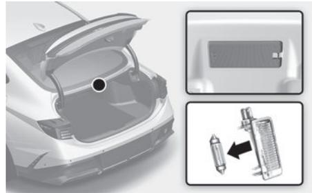
1. Using a flat-head screwdriver, gently pry the lens from the interior light housing.
