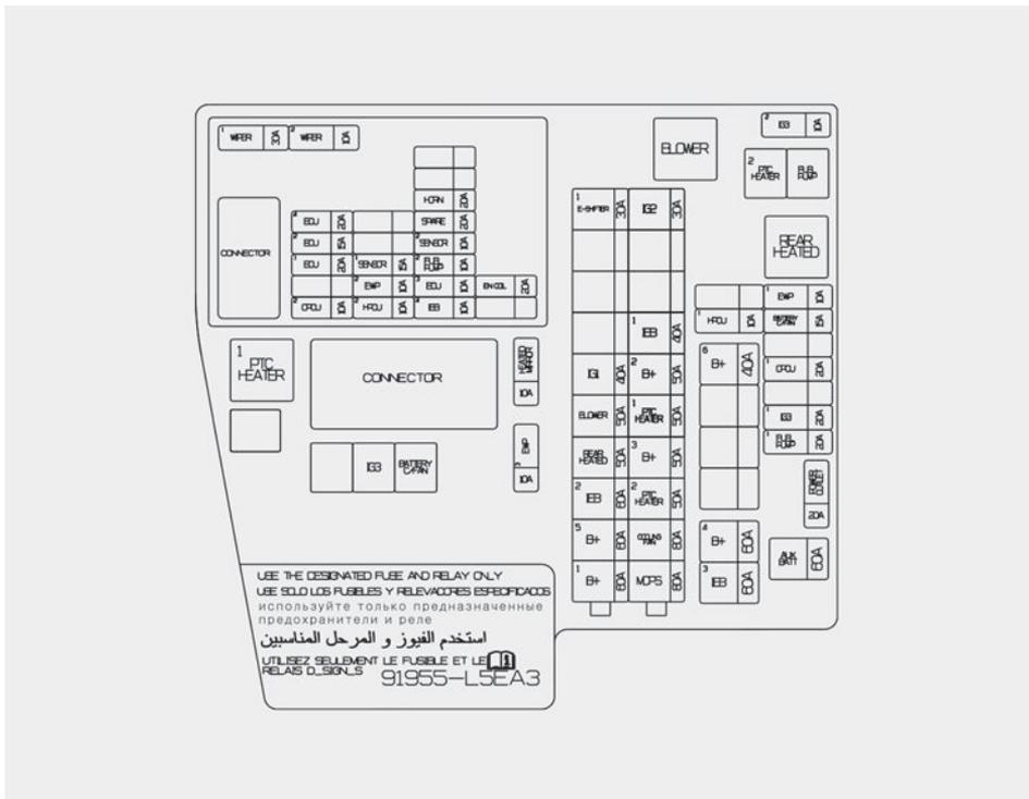
**Engine compartment fuse panel (Engine compartment junction block)**
