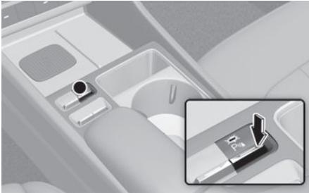
Press the Parking Safety (P<sup>W</sup>) button to turn on Parking Distance Warning. Press the button again to turn off the function.
