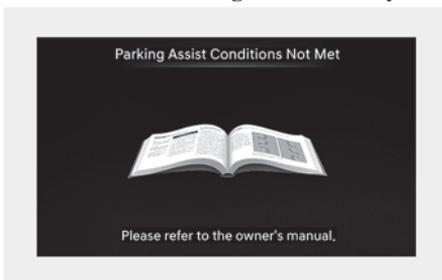
The **"Parking Assist Conditions not met"** message appears when Parking/View (P) button has been pressed and held while Remote Smart Parking Assist is in standby. After a while, press and hold the Parking/View (P) button again to see if Remote Smart Parking Assist works. The message appears even when the smart key's battery is low. Check the smart key battery level.
