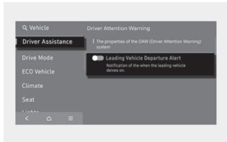
With the engine on, select **Setup > Vehicle > Driver Assistance > Driver Attention Warning** and then enable **Leading Vehicle Departure Alert** in the infotainment system to use the function.
