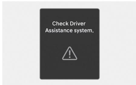
When Safe Exit Warning is not working properly, the "**Check Driver Assistance system.**" warning message will appear on the instrument cluster for several seconds, and the master warning light (
