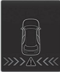
When the Rear Cross-Traffic Collision-Avoidance Assist is operating, if the function is not working normally or the radar is blocked, the master warning light (
