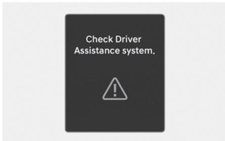
When Lane Keeping Assist is not working properly, the "**Check Driver Assistance system.**" warning message and yellow Lane Keeping Assist (
