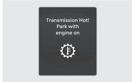
Repeated sudden acceleration and quick start may overheat the transmission. If the transmission is overheated, the self-protection mode alarms the driver with an audible sound warning message.
