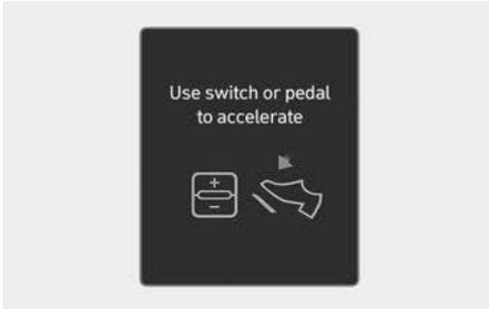
When Highway Driving Assist is operating, your vehicle will stop if the vehicle ahead of you stops. Also, if the vehicle ahead of you starts moving within 30 seconds after the stop, your vehicle will start as well. In addition, after the vehicle has stopped and 30 seconds have passed, the **"Use switch or pedal to accelerate"** message will appear on the instrument cluster. Depress the accelerator pedal or operate the + switch, - switch or (II) switch to start driving.
