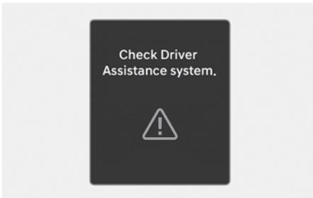
When Highway Driving Assist is not working properly, the "**Check Driver Assistance system.**" warning message and yellow Lane Keeping Assist (/⊕\) warning light appears on the instrument cluster. If this occurs, have your vehicle inspected by an authorized HYUNDAI dealer.
