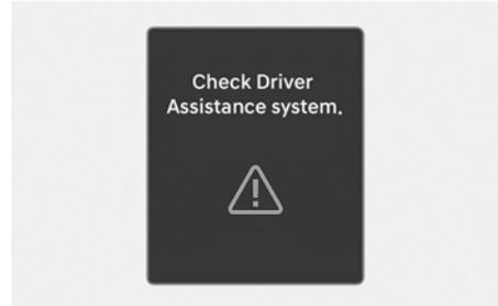
When Intelligent Speed Limit Assist is not working properly, the "**Check Driver Assistance system.**" warning message will appear on the instrument cluster for several seconds, and the master (⚠) warning light and speed limit (⊞) warning light will appear on the instrument cluster. If this occurs, have your vehicle inspected by an authorized HYUNDAI dealer.
