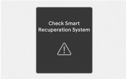
If the rear radar is covered by any foreign material, such as snow, rain, or dirt, the detecting performance may decrease and disable the smart recuperation system.
