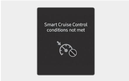
If the Driving Assist button, + switch, - switch or (II) switch is operated when Smart Cruise Control operating conditions are not satisfied, the "**Smart Cruise Control conditions not met**" will appear on the instrument cluster, and an audible warning will sound.
