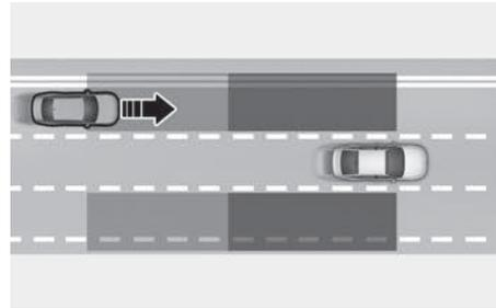
Blind-Spot Collision-Avoidance Assist helps detect and informs the driver that a vehicle is approaching at high speed from the blind spot area.
