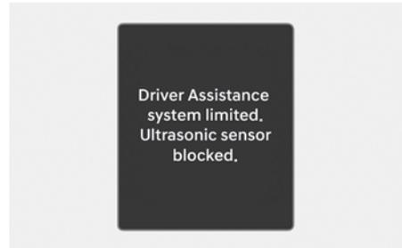
If this occurs the **"Driver assistance system limited. Ultrasonic sensor blocked"** warning message appears on the instrument cluster. Parking Distance Warning operates properly when snow, rain or foreign material is removed. If Parking Distance Warning does not operate properly after obstruction (snow, rain, or foreign material) is removed (including trailer, carrier, etc., from the rear bumper), have your vehicle inspected by an authorized HYUNDAI dealer.
