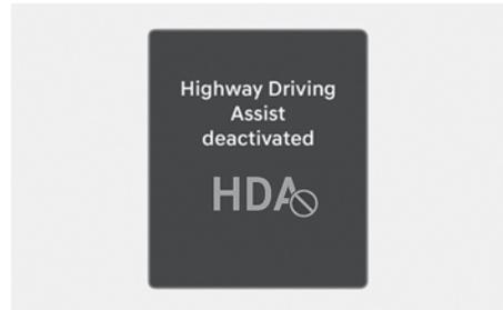
If the driver still does not have their hands on the steering wheel after the hands-off warning, **"Highway Driving Assist deactivated"** warning message will appear and Highway Driving Assist will be automatically canceled.
