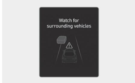
In the following situation, the "**Watch for surrounding vehicles**" warning message will appear on the instrument cluster, and an audible warning will sound to warn the driver of road conditions ahead.
