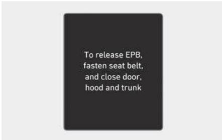
If the driver's seat belt is unfastened, or the hood, trunk, doors are open, and you try to drive with EPB applied, a warning sounds and a message appears.
