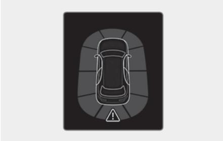
A master warning light (△) appears in the relative directions in case of a malfunction or blinding of the ultrasonic sensors while the Reverse Parking Collision-Avoidance Assist (PCA) is active. You can check the message in the utility information view of the instrument cluster.
