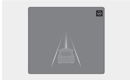
If the vehicle ahead and/or both lane markings are detected and your vehicle speed is below 120 mph (200 km/h), the green (⊕) indicator light appears on the instrument cluster, and Lane Following Assist helps center the vehicle in the lane by assisting the steering wheel.
