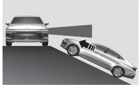
Rear Cross-Traffic Collision-Avoidance Assist may be limited when the vehicle is on an uphill or downhill slope, or near it, and may not detect the vehicle approaching from the left or right. If this occurs, the function may not warn the driver or control the brakes when necessary.
