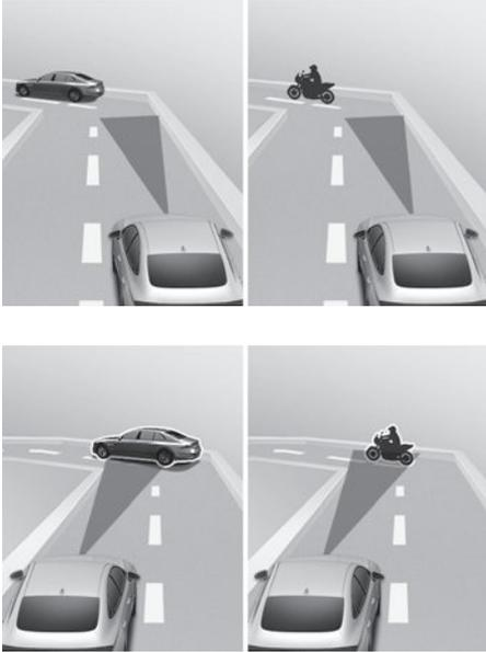
On curves, the smart recuperation system may not detect a vehicle in the same lane, and may accelerate the vehicle by lowering the regenerative braking intensity automatically. Your vehicle speed may decelerate by increasing regenerative braking intensity automatically if a vehicle is detected in an adjacent lane or when a vehicle ahead is detected suddenly. Apply the brake pedal or accelerator pedal depending on the road and driving conditions.
