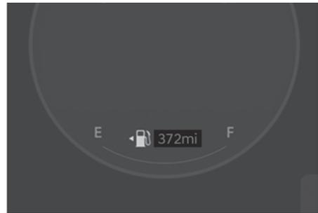
The distance to empty is the estimated distance the vehicle can be driven with the remaining fuel.
