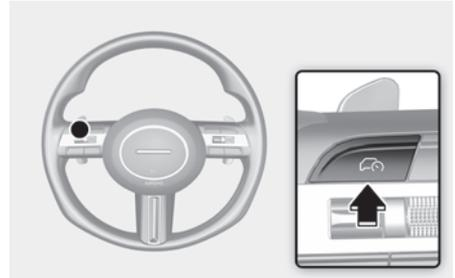
2. Push the + switch up or - switch down, and release it at the desired speed. Push the + switch up or - switch down and hold it. The speed will increase or decrease to the nearest multiple of 5 (multiple of 10 in km/h) at first, and then increase or decrease by 5 mph (10 km/h).
