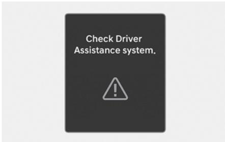
When Forward Collision-Avoidance Assist is not working properly, the "**Check Driver Assistance system.**" warning message will appear, and the (⚠), (🚫) warning light will illuminate on the instrument cluster. Have your vehicle inspected by an authorized HYUNDAI dealer.
