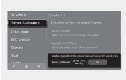
With the engine on, select or deselect **Setup > Vehicle > Driver Assistance > Speed Limit** from the Settings menu to set whether to use each function.
