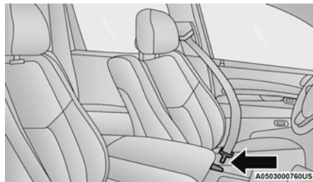
Inserting Latch Plate Into Buckle
