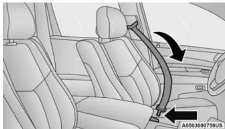
Pulling Out The Latch Plate
