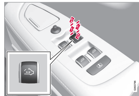
Panoramic roof control.
