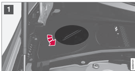
Coolant expansion tank, left-hand drive vehicle.
