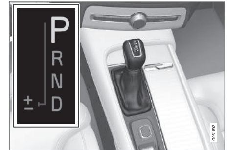
Overview of large gear selector and gear shift pattern in the instrument panel
