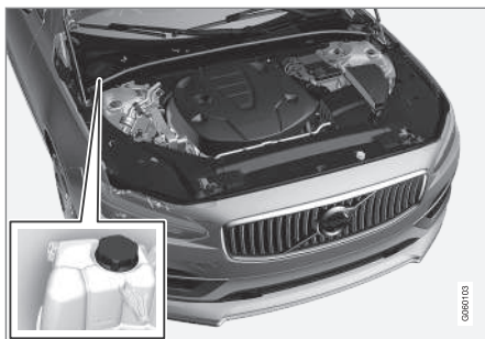
Coolant expansion tank, left-hand drive vehicle.
