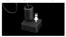
Let the compressor run for max. 10 minutes to fill the tire with sealing compound and achieve a tire inflation pressure of approx. 2.5 bar.
