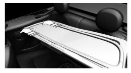
3. To release the lock, fold the handle up and hold it.
