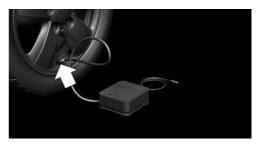
3. Insert the connector into the power socket in the vehicle interior.
