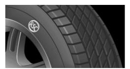
Runflat tires are labeled with a circular icon containing the letters RSC marked on the tire sidewall.
