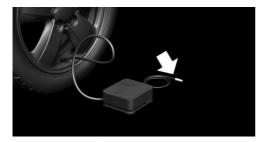
With the ignition turned on or the engine running, turn on the compressor and let it run for a maximum of 10 minutes.
