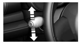
Press the lever past the resistance point. Canada: the lever returns into its initial position after actuation. To switch off manually, slightly tap the lever to the resistance point.
