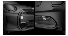
Threaded holes for the tow fitting are located in the front and rear of the vehicle on the right side with respect to the driving direction.
