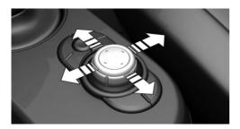
Without navigation system: tilt in two directions to switch between displays, for example.
