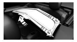
Press the wind deflector downward in the middle, until the handle engages, arrows 1.
