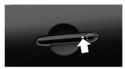
Press and hold down the button on the external door handle of the driver's or front passenger door.
