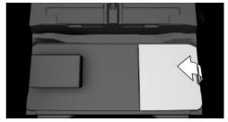
Located under the cargo floor panel on the right side is a recess for the onboard vehicle tool kit.
