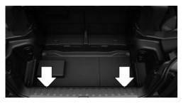
To secure the cargo there are two lashing eyes in the cargo area.
