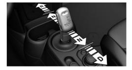
The selector lever positions R, N, and D are selected by tapping the selector lever forward or back. The selector lever automatically returns to the center position when released.
