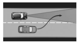
A vehicle driving in front of you is not detected until it is completely within the same lane as your vehicle.
