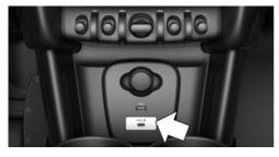
Depending on the equipment version, a USB port Type A or a USB port Type A and a USB port Type C are located in the front of the center console.
