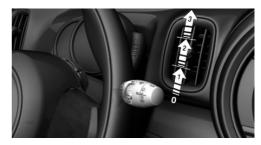
To activate: press the lever up once from its basic setting, arrow 1.
