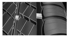
Distributed over the tire circumference are the tire manufacturer's wear indicators with a height of at least 0.06 in/1.6 mm, which serve as an indicator of tire tread wear.
