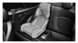
The rear seat belts and the front passenger seat belt can be permanently locked to fasten child restraint systems.
