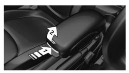
Press button, arrow 1, and open center armrest upward, arrow 2.
