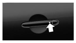
Press the button on the door handle of the driver's or front passenger door.
