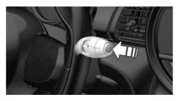
Press the button on the wiper lever.
