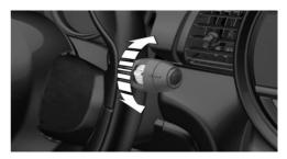
Turn the thumbwheel on the wiper lever.
