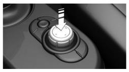
With navigation system: tilt in four directions to switch between displays, for example.
