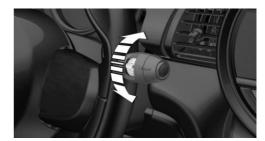
Turn the thumbwheel on the wiper lever.
