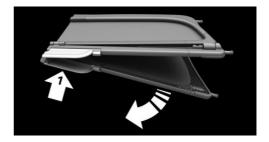
2. Open the rear side window, if necessary. Insert wind deflector from one side of the vehicle with the pins in the corresponding mounting points on the opposite side of the vehicle.
