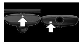
Photocells are used for control:
