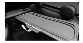
Press the wind deflector inwardly and up, arrow 1, to the extent that the wind deflector can be positioned in front of the mounting points on the installation side. Release the handle.
