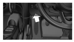
On the driver's side, there is a socket for onboard diagnosis to check components that are relevant for the vehicle's emission mix.
