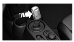
2. With the driver's seat belt fastened, briefly push the selector lever in the desired direction, past a resistance point, if needed. The selector lever automatically returns to the center position when released.
