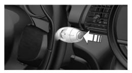
Press the button on the wiper lever.
