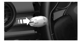
Reset the current travel time: press button on the turn signal lever for approx. 2 seconds with the travel times displayed.
