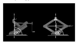
6. Make sure that the car jack foot stands vertically and perpendicularly beneath the jacking point after extending the vehicle jack.
