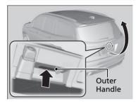
When all the doors are unlocked or press the tailgate unlock button on the remote transmitter, the tailgate is unlocked. Press the tailgate outer handle and lift open the tailgate.
