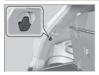
The cargo hooks on both sides of the cargo area can be used to hang a light items.
