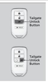
Press the tailgate unlock button to unlock the tailgate.
