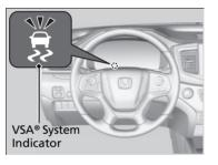
When VSA<sup>®</sup> activates, you may notice that the engine does not respond to the accelerator. You may also notice some noise from the hydraulic brake system. You will also see the indicator blink.
