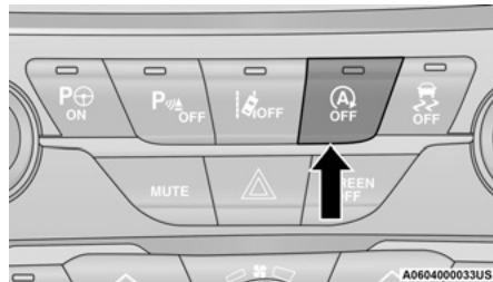
Stop/Start OFF Switch
