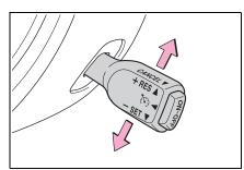
At this time, the Conventional Cruise Control indicator (green) is illuminated in the meter. The set speed will be shown on the meter. You can change the displayed units by operating the meter display. (→P.400)
