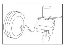
9 Adjust the air pressure to the appropriate level (green zone of the air gauge).
