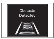
Vehicles in front in the same traffic lane are detected by the stereo camera within a distance of approximately 360 ft (110 m) in the forward direction. However the detection distance may be reduced depending on the traffic environment, driving conditions, and conditions of the vehicle in front.
