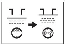
If the "UPPER LEVEL" line cannot be seen, check the fluid level by looking directly at the cell.
