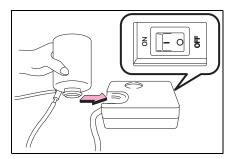
Make sure that the air compressor switch is off.
