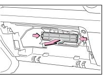
6 Remove the air conditioning filter and replace it with a new
