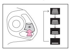
The following distance changes corresponding with the vehicle speed. The faster the vehicle travels, the greater the following distance.
