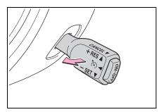
To resume the Conventional Cruise Control after it has been temporarily canceled and with vehicle speed of approximately 20 mph (30 km/h) or more, push the lever up to return to the original cruising speed automatically.
