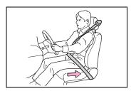
Do not sit or lean close to either door. The SRS side airbags are stored in both front seat seatbacks next to the door, and they provide protection by deploying rapidly in the event of a side impact collision. However, the force of SRS side airbag deployment can injure an occupant whose body is too close to an SRS airbag.
