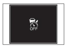
● If EyeSight is malfunctioning, (yellow) is displayed on the meter display, and the Pre-Collision Braking System OFF indicator and Lane Departure Warning OFF indicator illuminate. If this occurs, stop the vehicle in a safe location and then turn off the engine and restart it. If the indicators remain illuminated after restarting the engine, Adaptive Cruise Control
