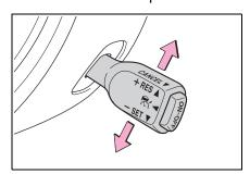
When Adaptive Cruise Control is activated, "READY" indicator turns off, the set vehicle speed is displayed, and 🛣 changes
