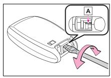
3 Remove the depleted battery.
