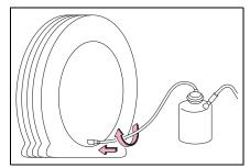
5 Turn the bottle upside down and tilt the bottle cap into the bottle holder of the air compressor.
