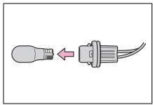
5 Install a new light bulb then install the bulb base to the light unit by inserting it and
