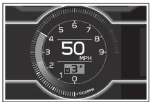
The engine speed at which the REV indicator is displayed can be changed on 💢 of the multi-information display. (→P.400)
