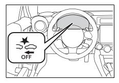
When the Pre-Collision Braking System OFF indicator is turned on, Pre-Collision Braking System (including the Pre-Collision Braking Assist function) and Pre-Collision Throttle Management do not oper-
