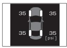
If the tire pressure drops below a predetermined level, the driver is warned by a screen display and a warning light. (→P.354)
