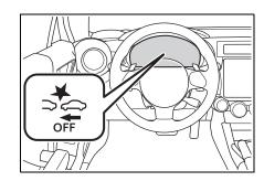
When the Pre-Collision Braking System OFF indicator is turned on, Pre-Collision Braking System (including the Pre-Collision Braking Assist function) and Pre-Collision Throttle Management do not operate. 4
