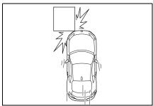
Examples of the types of accidents in which it is possible that the SRS side airbag and the SRS curtain shield airbag will deploy. It is possible that the SRS side and curtain shield airbags will deploy if a serious impact occurs to the underside of your vehicle. Some examples are shown in the illustration.
