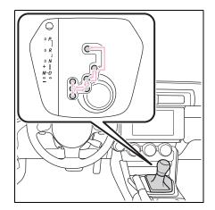
While the engine switch is in ON, move the shift lever with the brake pedal depressed.
