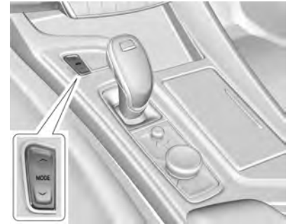
Driver Mode Control Switch
