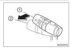
The headlight high-beam indicator light in the combination meter illuminates simultaneously. The lever will return to the normal position when released.
