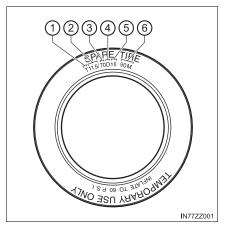
T115/70D16 90M is an example of a tire size and load index rating. Here is an explanation of the various components of that tire size and load index rating. Note that the tire size and load index rating may be different from the example.
