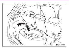
Thread the buckle through the wheel as shown in the figure.
