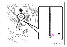
Use plain water if washer fluid is unavailable. But use only washer fluid in cold weather to prevent it from freezing.
