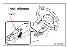
3 Attempt to push the steering wheel up and down to make sure it's locked before driving.
