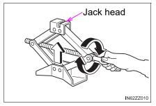
5 Place the jack under the jackup position closest to the tire being changed with the jack head squarely under the jackup point.
