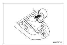
To return to automatic shift mode, shift the lever from M to D.
