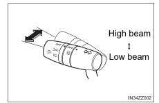
When the headlight high-beams are on, the headlight high-beam indicator light is turned on.
