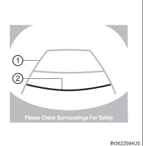
The red and yellow lines indicate the points about 19 in. (500 mm) for the red line and 39.3 in. (1000 mm) for the yellow lines from the rear bumper (at the center point of each of the lines).
