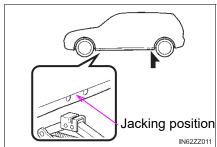
6 Continue raising the jack head gradually by rotating the screw with your hand until the jack head is inserted into the jack-up position.
