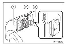
If it is at or near L, add enough coolant to the coolant reservoir to provide freezing and corrosion protection and to bring the level to F. Securely tighten the coolant reservoir tank cap after adding coolant.
