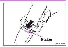
If a belt does not fully retract, inspect it for kinks and twists. If it is still not retracting properly, have it inspected at your Toyota dealer.
