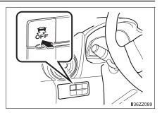
Press the switch again to turn the TCS/DSC back on. The DSC OFF indicator light will turn off.
