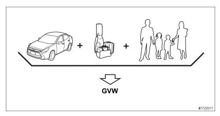
GVW (Gross Vehicle Weight) is the Vehicle Curb Weight + cargo + passengers.
