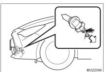
5 Turn the socket and bulb assembly to remove it. Carefully remove the bulb from its socket in the reflector by gently pulling it straight backward out of the socket.
