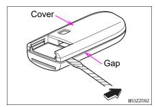
Twist the flathead screwdriver in the direction of the arrow and remove the cover.
