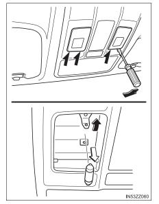
3 Install the new bulb in the reverse order of the removal procedure.
