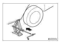
Turn the jack handle clockwise and raise the vehicle high enough so that the spare tire can be installed. Before removing the lug nuts, make sure your Toyota is firmly in position and that it cannot slip or move.
