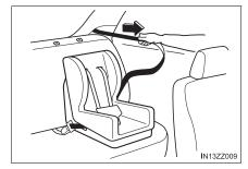
Fush the child-restraint system firmly into the vehicle seat. Be sure the belt retracts as snugly as possible. A clicking noise from the retractor will be heard during retraction if the system is in the automatic locking mode. If the belt does not lock the seat down tight, repeat this step.
