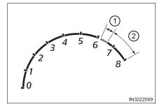
When the tachometer needle enters the STRIPED ZONE, this indicates to the driver that the gears should be shifted before entering the RED ZONE.
