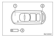
To use the auxiliary key, press the knob and pull out the auxiliary key from the smart key.
