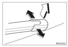
2 Remove the stopper and raise the wiper arm.
