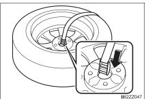
14 Thread the belt through the buckle while pressing the tire to the seatback.
