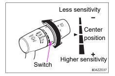
From the center position (normal), rotate the switch upward for higher sensitivity (faster response) or rotate it downward for less sensitivity (slower response).
