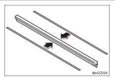
6 Carefully insert the new blade rubber. Then install the blade assembly in the reverse order of removal.
