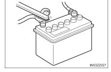
• If the vehicle will not be used for an extended time, disconnect the battery cables and charge the battery every 6 weeks.
