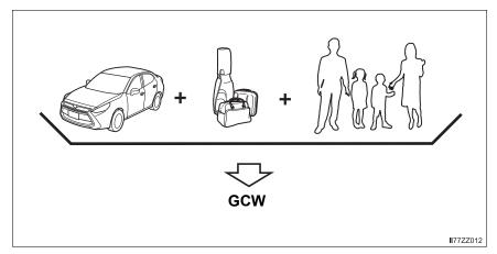
GCW (Gross Combination Weight) is the weight of the loaded vehicle (GVW).
