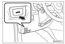
Using the electric trunk lid opener (With the advanced keyless function)
