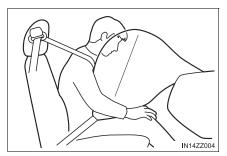
In addition, the front passenger air bag is designed to only deploy in accordance with the total seated weight on the front passenger seat. For details, refer to the front passenger occupant classification system ( $\rightarrow$ P. 82).
