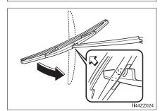
4 Pull down the blade rubber and slide it out of the blade holder.
