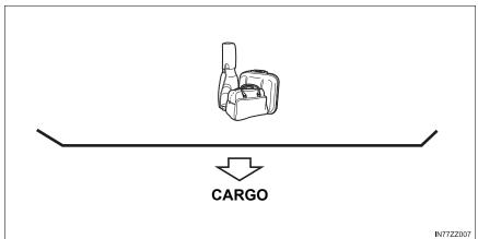
Cargo Weight includes all weight added to the Base Curb Weight, including cargo and optional equipment.
