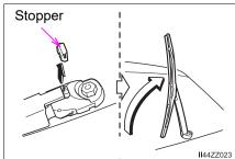
3 Firmly rotate the wiper blade to the right until it unlocks, then remove the blade.
