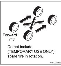
Inspect the tires for uneven wear and damage. Abnormal wear is usually caused by one or a combination of the following:
