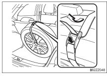
15 Pull the belt end to secure the flat tire.
