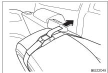
Insert the luggage compartment cover from the top of the luggage compartment opening with the cloth side of the cover facing outward, and slide it between the flat tire and the inside perimeter of the luggage compartment opening.
