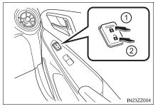
To lock all the doors and the liftgate from an open front door, press the lock side of the door lock switch and then close the door.
