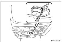
4 Using a flathead screwdriver, turn the lever to the right to unlock the liftgate.
