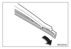
5 Remove the metal stiffeners from the blade rubber and install them in the new blade.
