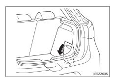
2 Turn the wing bolt and jack screw counterclockwise.
