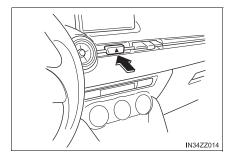
Depress the hazard warning flasher and all the turn signals will flash. The hazard warning indicator lights in the combination meter flash simultaneously.
