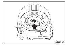
3 Turn the wing bolt and jack screw counterclockwise.
