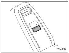
Passenger's window can be controlled by the power window switch located on the door.
