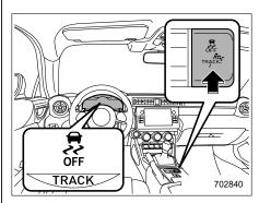
The TRACK indicator and Vehicle Stability Control (VSC) OFF indicator come on when in TRACK mode.
