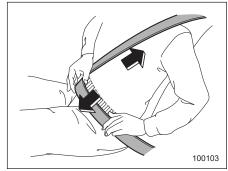
4. To tighten the lap part, pull up on the shoulder belt.
