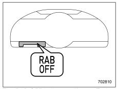
The RAB OFF indicator will turn off when the corresponding function is turned ON.
