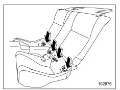
The lower anchorages (bars) are used for installing a child restraint system. For each seating position, two lower anchorages are provided. Each lower anchorage is located where the seat cushion meets the seatback.
