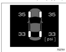
This screen displays each tire pressure. Refer to "Combination Meter Display (Color TFT)" \*P151.
