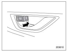
2. Rotate the lock lever forward.
