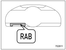
If the Reverse Automatic Braking (RAB) system malfunctions, the above indicator illuminates on the combination meter. Contact the nearest SUBARU dealer for details.
