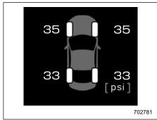
This screen displays each tire pressure. When a tire is deflated, the deflated tire and the tire pressure will be displayed on the screen in yellow.
