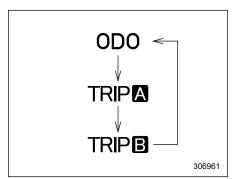
To reset the trip meter, select either the A trip or B trip meter, then press and hold the TRIP RESET switch.
