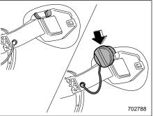
5. Set the fuel filler cap on the cap holder inside the fuel filler lid.
