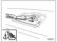
2. Fasten the top tether hook of the child restraint system to the appropriate upper anchorage.
