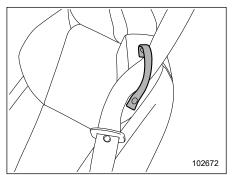
To enable the seatbelt to be easily extended, pass the seatbelt through the guide. When getting in or out of the rear seats, release the seatbelt from the guide.
