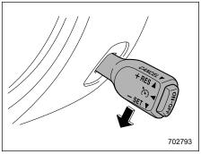
3. Press the Cruise control switch to the "-SFT" side and release it.
