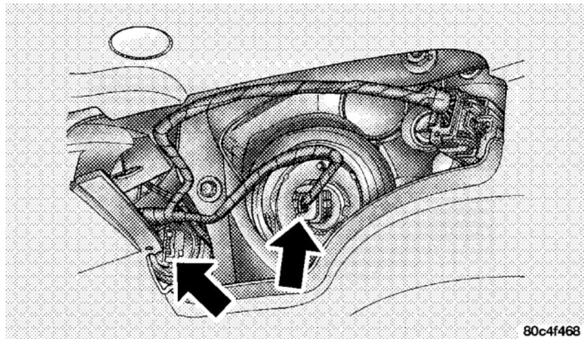
3. Rotate the socket to the left one-quarter turn, and replace the bulb.
