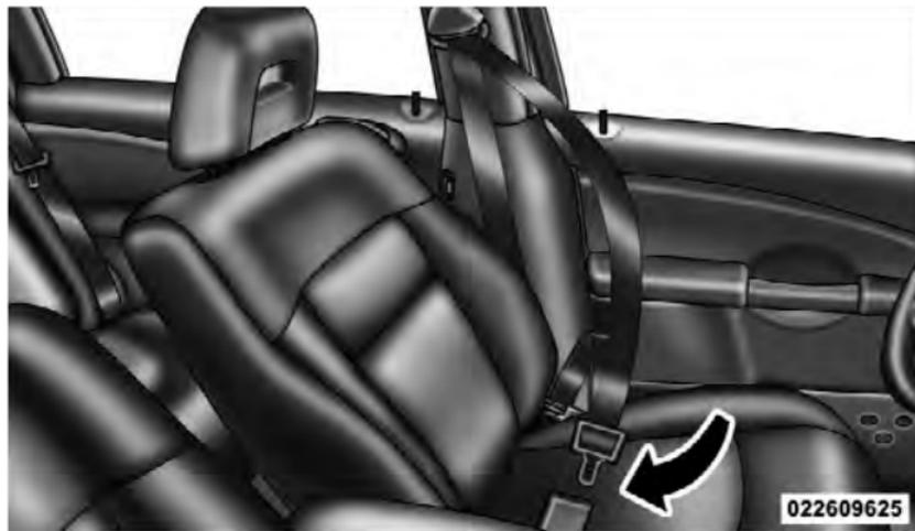
Inserting Latch Plate Into Buckle
