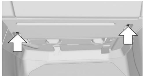
Loosen fasteners, arrows, and open cover.
