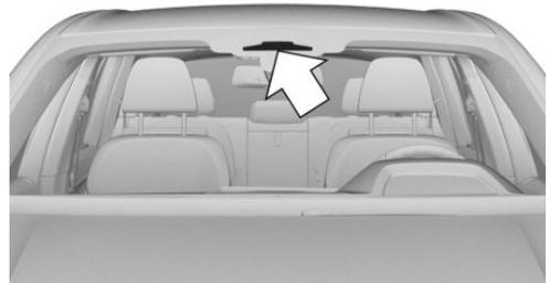
The cameras are located in the area of the interior mirror.
