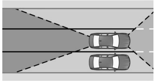
Radar sensors monitor the space next to the vehicle when traveling faster than a minimum speed of up to approx. 130 mph/210 km/h.
