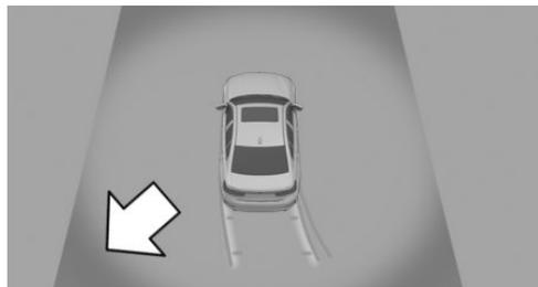
In the PDC Park Distance Control view, the respective boundary area flashes red, if vehicles are detected by the sensors.
