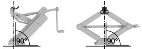
6. Make sure that the vehicle jack foot stands vertically and perpendicularly beneath the jacking point after extending the vehicle jack.
