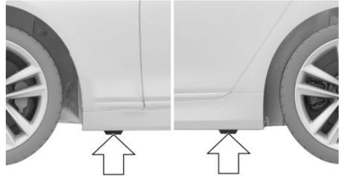
The jacking points for the vehicle jack are located at the indicated positions.
