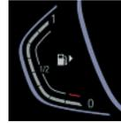
An arrow next to the fuel pump symbol indicates the vehicle side on which the fuel filler flap is located.
