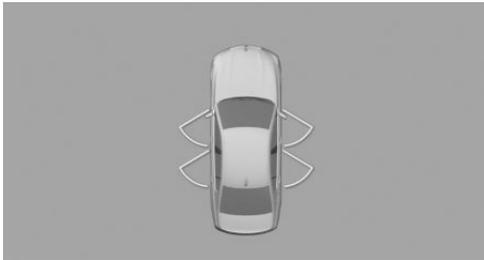
Steptronic transmission: the maximum opening angles of the doors are displayed in selector lever position P. As soon as the vehicle begins moving, the opening angles are replaced by parking aid lines.
