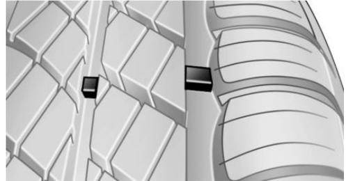
Wear indicators are distributed around the tire circumference. These wear indicators have the legally required minimum height of 0.063 in/1.6 mm.
