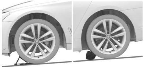
If you need to change a wheel on a slight downhill grade, place chocks and other suitable objects, for instance rocks, under the wheels of both the front and rear axles against the rolling direction.
