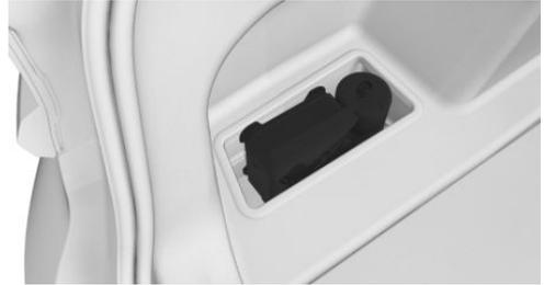
Storage for the tire repair set is provided in the left storage compartment of the trunk.
