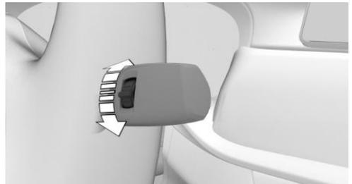
Turn the thumbwheel to adjust the sensitivity of the rain sensor.
