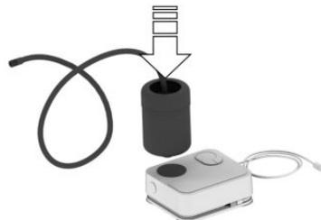
4. Screw the filler hose of the sealant bottle onto the tire valve of the nonworking wheel.
