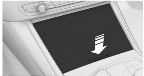
2. A socket is located between the cup holders. Pull off the cover.
