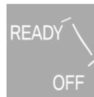
The letters OFF in the tachometer indicate that drive-ready state is switched off and standby state is switched on.
