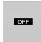
The lettering OFF in the instrument cluster indicates that drive-ready state is switched off and standby state is switched on.
