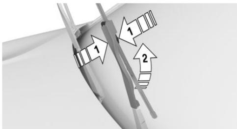
4. Remove the wiper blade forward from the catch.
