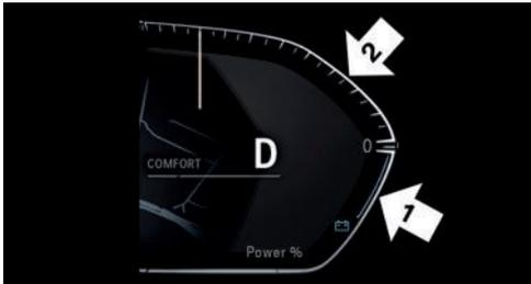
Pointer in the area of arrow 1: display of the energy recovered by coasting or when decelerating, CHARGE.
