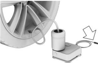
6. With standby state or drive-ready state switched on, switch on the compressor.
