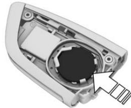
4. Insert a type CR 2032 3V battery with the positive side facing up.
