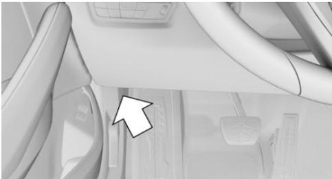
Located on the driver's side is an OBD socket for reading the vehicle data.
