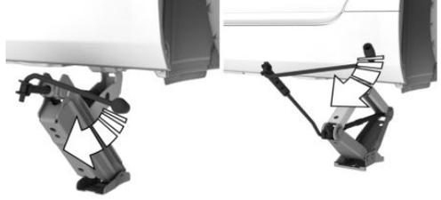
4. Take your hand away from the vehicle jack as soon as the vehicle jack is under load and continue turning the vehicle jack crank or lever with one hand.
