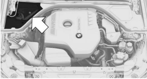
The battery for the Mild-Hybrid technology is located under a cover in the engine compartment on the front passenger side.
