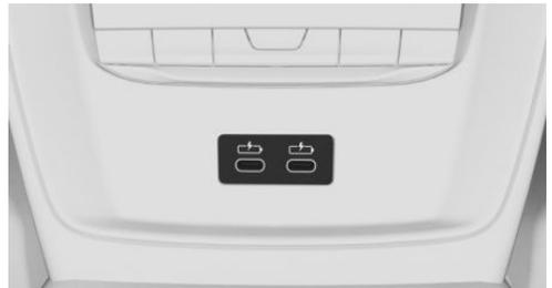
Two USB ports are located in the center console in the rear passenger compartment.
