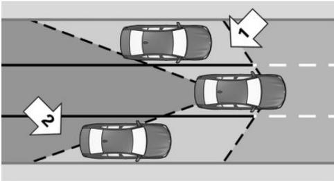
Radar sensors monitor the area behind and next to the vehicle when traveling faster than a minimum speed.
