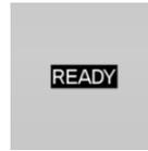
The letters READY in the instrument cluster indicate that the drive readiness is turned on and the Auto Start/Stop function is ready to start the engine automatically.
