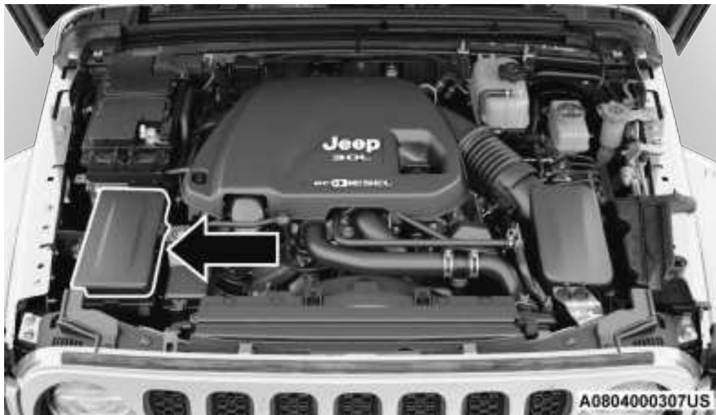
Power Distribution Center Location – Diesel Engine
