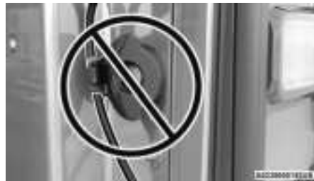
Incorrectly Seated Tailgate Strap
