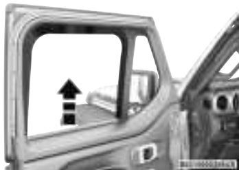
Push Upward On Middle Of Upper Half Door To Remove
