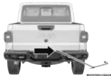
Inserting The Extensions Into The Winch Mechanism Access Hole
