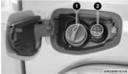
Fuel and Diesel Exhaust Fluid (DEF) Fill Location
