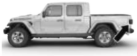
BSM Radar Location (Left Side Shown)
