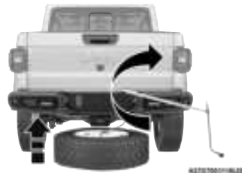
Reinstalling The Flat Or Spare Tire
