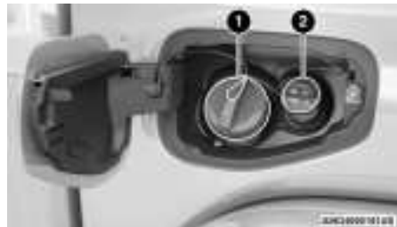
Fuel and Diesel Exhaust Fluid Fill Location
