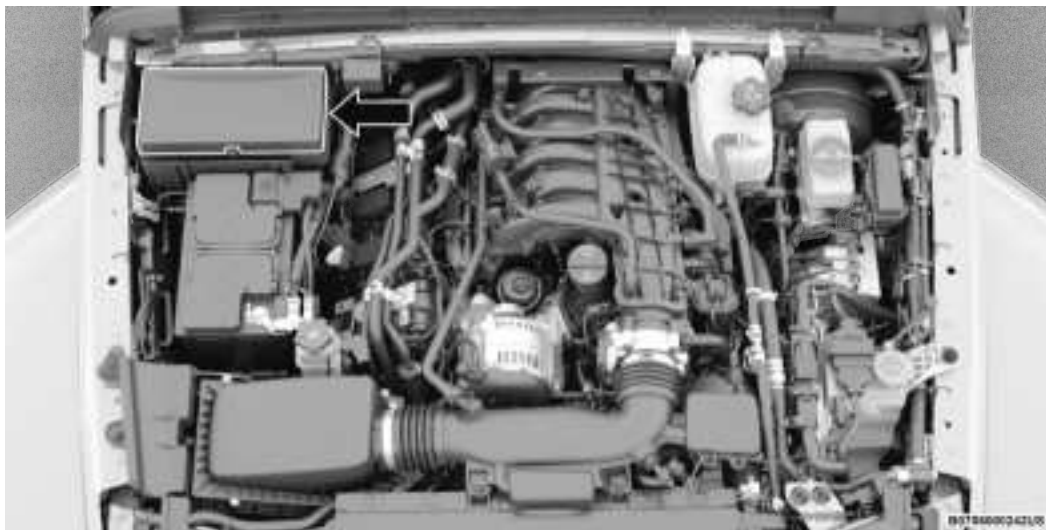
Power Distribution Center Location – Gas Engine
