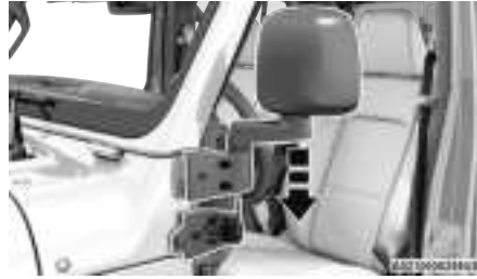
Lower Mirror Assembly Onto Bracket
