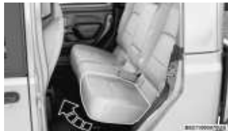
Lift From Beneath Seat (Left Side Shown)
