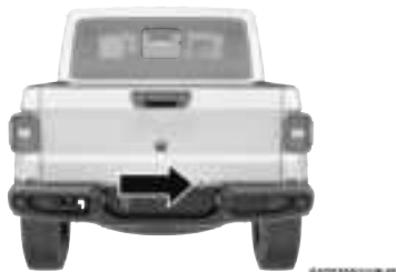
Access Hole Location
