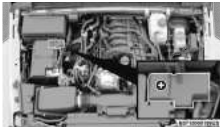
Positive (+) Battery Post – Gas Engine
