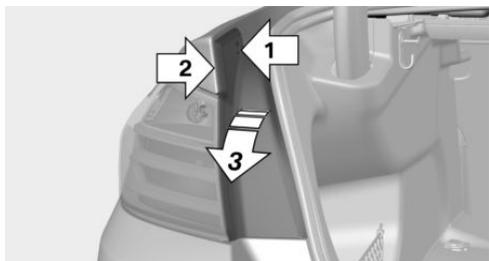
3. Use the screwdriver from the onboard vehicle tool kit to press in the latch, arrow 2, and remove the cover, arrow 3.
