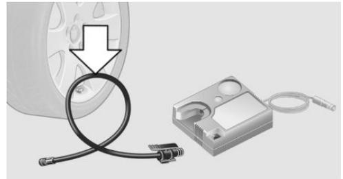
3. Attach the connection hose to the connector of the sealing container, ensuring that it engages audibly.
