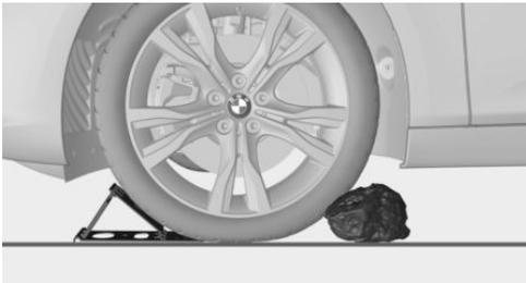
Place chocks or other suitable objects, for example a rock, in front of and behind the wheel that is diagonally opposite to the wheel that you wish to change.
