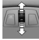
If there is an external danger, push the switch forward past the resistance point and hold it.
