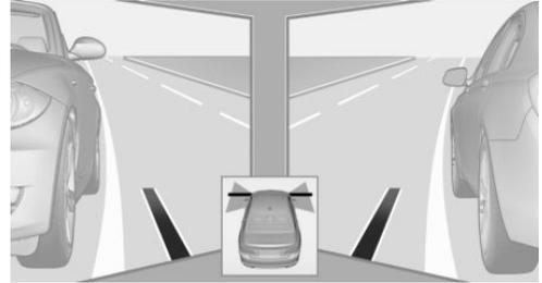
Guidelines at the bottom of the image show the position of the front of the vehicle.
