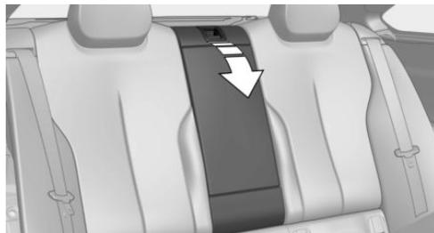
Reach into the recess and pull the middle section forward.
