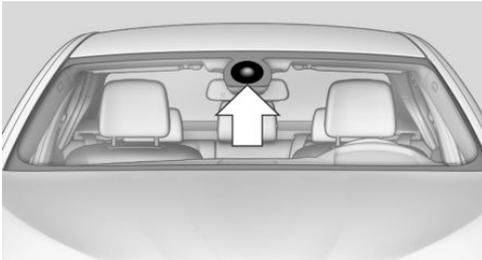
The camera is installed near the interior mirror. Keep the windshield in front of the interior mirror clean and clear.
