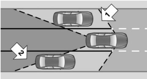
Two radar sensors in the rear bumper monitor the area behind and next to the vehicle at speeds above approx. 30 mph/50 km/h.
