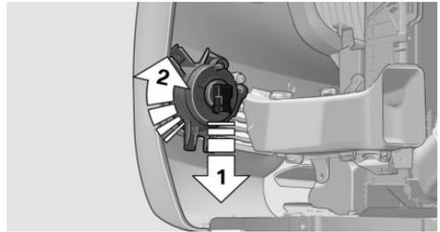
3. Insert the new bulb, connect the connector and screw on the wheel house panel.
