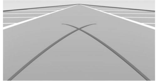
Turning radius lines can only be superimposed on the rearview camera image together with pathway lines.
