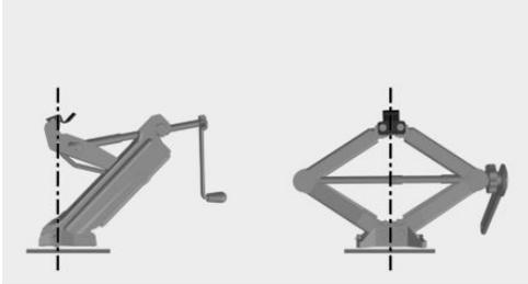
5. Make sure that the vehicle jack foot stands vertically and perpendicularly beneath the jacking point after extending the vehicle jack.
