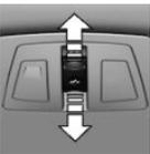
1. Press the switch forward beyond the resistance point and hold.
