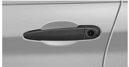
Unlock or lock the driver's door via the door lock using the integrated key.
