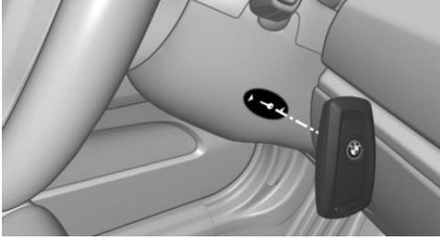
1. Hold the remote control with its back against the marked area on the steering column.
