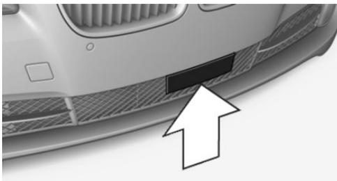
Always keep radar sensor clean and unobstructed.
