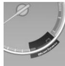
The energy of motion of the vehicle is converted to electrical energy while coasting. The vehicle battery is partially charged and fuel consumption can be reduced.
