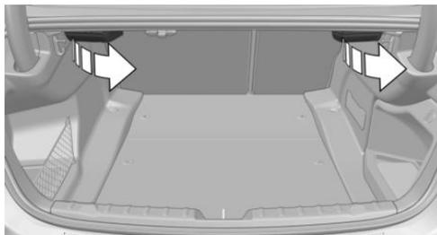
2. The unlocked backrest moves forward slightly.
