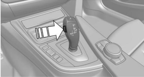
To release the lock: press button, arrow.
