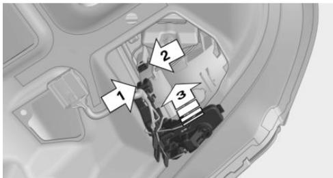
2. Press on the bulb holder, arrow 3. Make sure that the two exterior holders latch into place.
