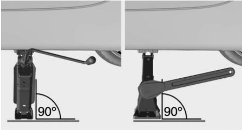
6. Crank up the vehicle jack until the entire surface of the jack is in contact with the ground and the wheel in question is raised a maximum of 1.2 inches/3 cm off the ground.
