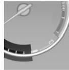
Displays the current fuel consumption. Check whether you are currently driving in an efficient and environmentally-friendly manner.
