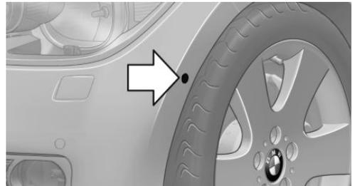
The four ultrasound sensors for measuring parking spaces are located in the front and rear on the side of the vehicle.
