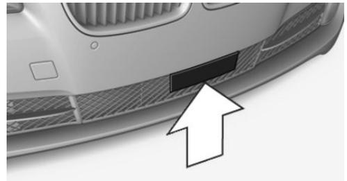
Always keep radar sensor clean and unobstructed.
