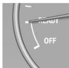
The READY display in the tachometer signals that the Auto Start/Stop function is ready to start the engine automatically.
