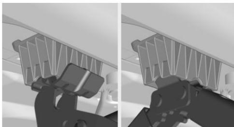
3. Extend the vehicle jack by turning the crank clockwise.
