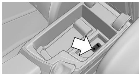
The USB interface and the AUX-IN port are located in the center armrest.
