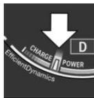
The mark in the efficiency display below the tachometer is backlit in blue and is located at the zero point. The tachometer approximately indicates idle
