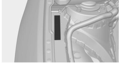
The vehicle identification number can be found in the engine compartment.
