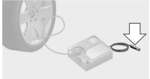
5. Correct the tire inflation pressure to 2.5 bar.
