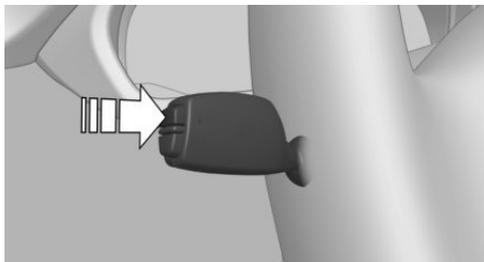
Press and hold button on signal lever.
