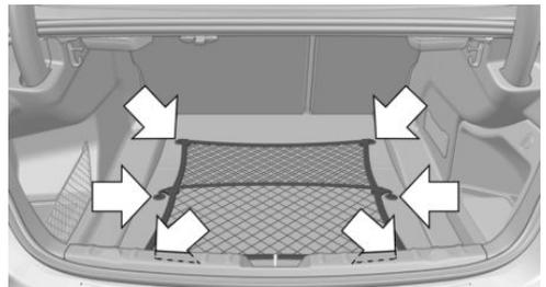
Hook the floor net into the fittings in the cargo area floor.
