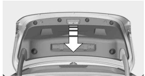
4. Press together hinge trim, see arrow, to release the clips.
