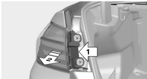
6. Release the catch at the top on the connector of the connecting line and remove the connector from the bulb holder.
