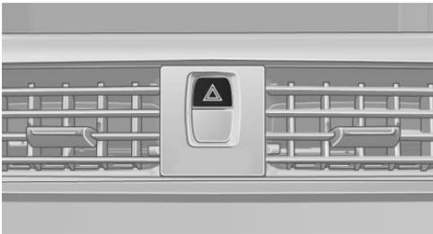
The button is located in the center console. The red lamp in the button flashes with the hazard warning flashers switched on.
