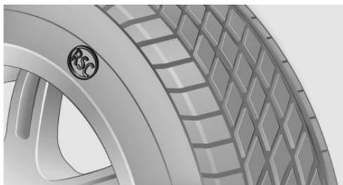
RSC label on the tire sidewall.
