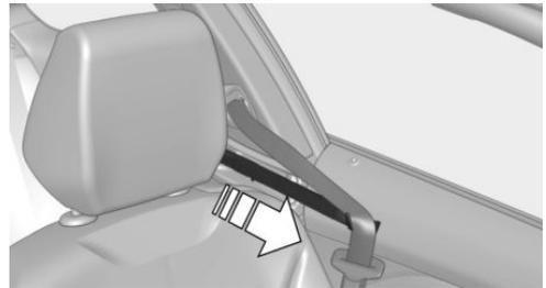
After the door is closed and the vehicle key has been detected in the vehicle's interior, the belt carrier extends automatically and keeps the safety belt ready to put on, arrow. After the belt is put on, it goes back into the idle position.
