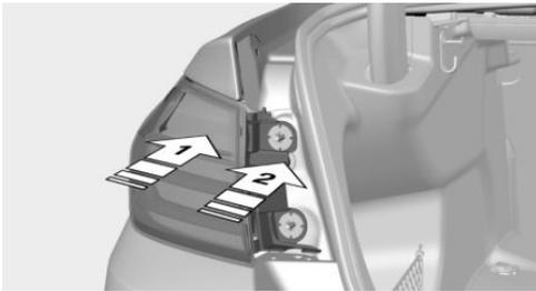
4. Screw the tail lamp on with the two nuts.
