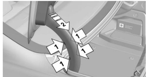
5. Carefully loosen the trim from the tailgate, starting at the edge and working toward the area around the recessed grips. Make sure that the trim does not become stuck.
