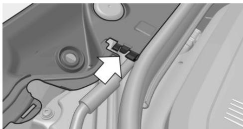
3. Press down on the holder and tighten the three screws.
