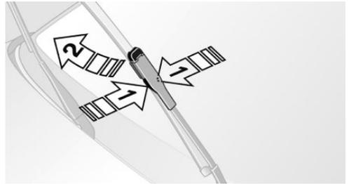
4. Remove the wiper blade forward from the catch.
