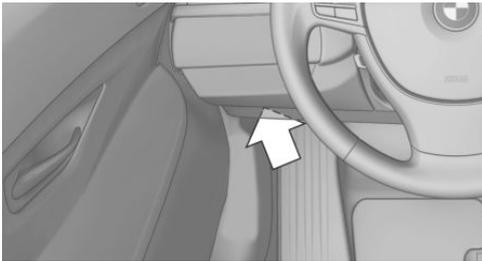
There is an OBD socket on the driver's side for checking the primary components in the vehicle's emissions.
