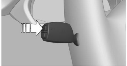
Press and hold button on signal lever.
