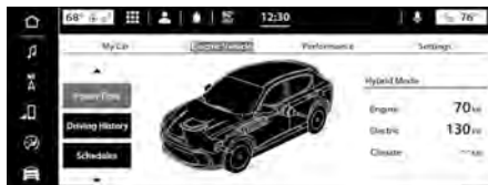
Power Flow Screen
