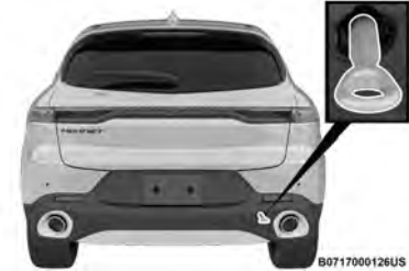
Rear Tow Eye Installed
