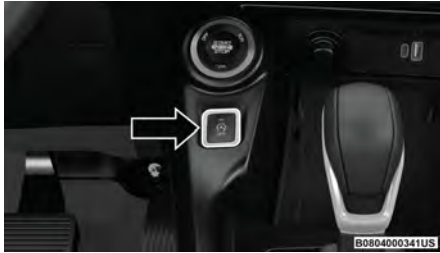
Stop/Start OFF Switch
