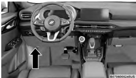
Interior Fuse Box Location
