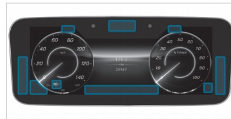
Driver's display with driver camera
