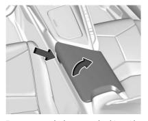
To open, press the button on the driver side. Depending on the options, there may be two USB ports and an auxiliary port inside.
