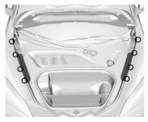
1. Release the four clips for the left and right outer covers.
