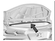
Use the pull cup to close the hatch/trunk with light force until the power latch feature activates. The hatch/trunk will close the rest of the way and latch automatically.
