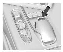
To activate My Mode, Weather, Tour, Sport and Track Mode, turn the Driver Mode Control (DMC) knob on the center console to make a mode selection. When a mode is selected, an indicator will come on in the instrument cluster and stay on.
