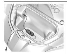
Some vehicles have a battery maintainer package. Follow the instructions provided with the battery maintainer package to keep the battery charged when the vehicle is not in use. Plug the battery maintainer into the underhood accessory power outlet only.
