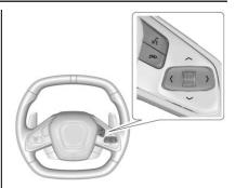
Press  $\leq$  or > to access the cluster applications. Use the thumbwheel to scroll  $\land$  or  $\lor$  through the list of available features. Press the thumbwheel to select. Not all applications will be available on all vehicles.
