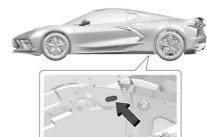
Use only a service jack with a lifting pad diameter of 64 mm (2.5 in) or smaller, and thick enough to make sure the jack does not contact the vehicle body.
