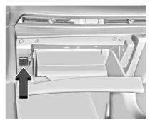
The PDR records video, audio, and vehicle data. The forward facing video and cabin audio are captured by a camera and microphone located behind the rear view mirror. The PDR video and data is stored on a removable SD card located in the SD card reader in the glove box. The video (MP4) can be played back in the vehicle or the SD card can be removed and played in a PC or on a mobile device or the file can be viewed and analyzed within Toolbox. See Toolbox later in this section.
