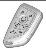
i: Press to lock both doors and the fuel door. The turn signal indicators may flash and/or the horn may sound on the second press to indicate locking. To view available settings from the infotainment screen, touch Settings > Vehicle > Remote Lock, Unlock, Start.
