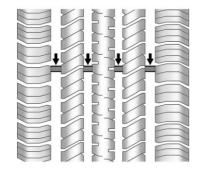
Treadwear indicators are one way to tell when it is time for new tires. Treadwear indicators appear when the tires have only 1.6 mm (1/16 in) or less of tread remaining. See *Tire Inspection* ⇒ 283 and *Tire Rotation* ⇒ 283.
