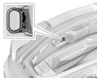
There is a glow-in-the-dark emergency hatch/trunk release handle on the inside back wall of the storage compartment. This
