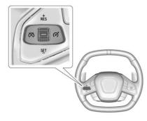
: Press to turn cruise control on or off. A white indicator comes on in the instrument cluster when cruise is turned on.
