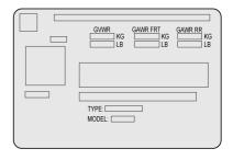
A vehicle-specific Certification label is attached to the rear edge of the driver door. It may show the gross weight capacity of the vehicle, called the Gross Vehicle Weight Rating (GVWR). The GVWR includes the weight of the vehicle, all occupants, fuel and cargo.
