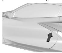
For Keyless Access, hold the remote key within 1 m (3 ft) of the door handle. Grip and press the door handle touchpad. See Remote Key Operation
