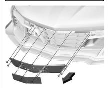
For Z06 vehicles only, remove the front license plate and bracket (if installed) and remove the front aero covers before track use. See your dealer for complete procedure.
