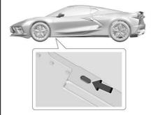
Use only a service jack with a lifting pad diameter of 64 mm (2.5 in) or smaller, and thick enough to make sure the jack does not contact the vehicle bodu.
