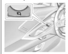
If equipped, press a to power fold the mirrors. Press again to unfold.
