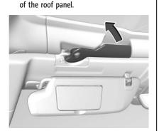
6. To unlock the front release handles, pull them outward, turning fully.
