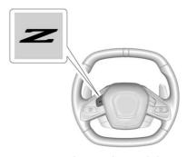
To activate Z-Mode, press the Z-Mode button on the steering wheel. To deactivate, select a different mode through the DMC knob, or press the Z-Mode button on the steering wheel.
