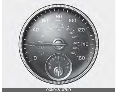
The speedometer indicates the speed of the vehicle and is calibrated in miles per hour (mph) and/or kilometers per hour (km/h).
