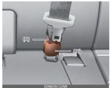
3. Pull out the tongue plate (B) from the pocket. Pull the tongue plate (B) and insert it into the buckle
