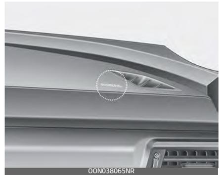
The indication of the system's presence are the letters "AIR BAG" located on the air bag pad cover on the steering wheel and the passenger's side front panel pad above the glove box.
