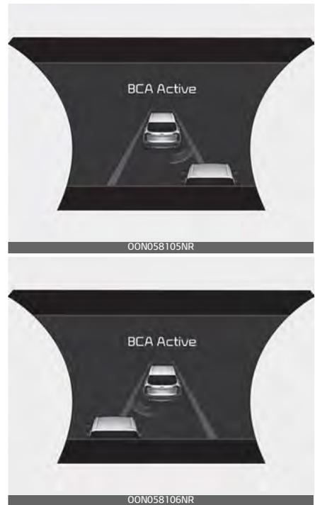
Blind-Spot Collision-Avoidance Assist may apply braking power, when an approaching vehicle is detected within a certain distance next to/behind your vehicle.
