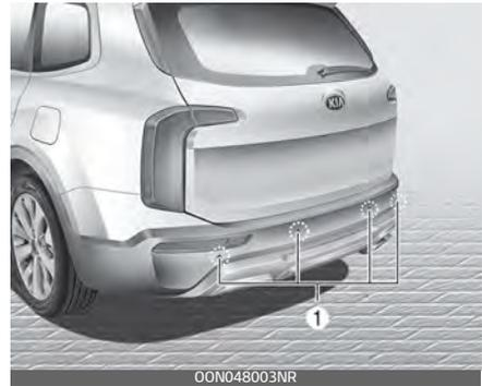
This function is a supplemental system and it is not intended to nor does it replace the need for extreme care and attention of the driver. The sensing range and objects detectable by the back sensors (1) are limited. Whenever backing-up, pay as much attention to what is behind you as you would in a vehicle without Reverse Parking Distance Warning.
