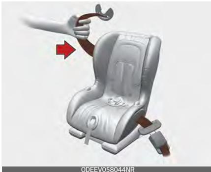
5. Remove as much slack from the belt as possible by pushing down on the CRS while feeding the shoulder belt back into the retractor.
