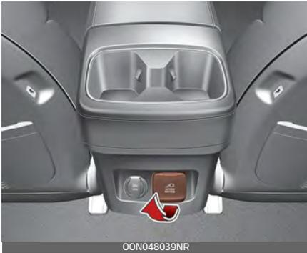
The AC inverter supplies 115 V / 150 W electric power to operate electric accessories or equipment.
