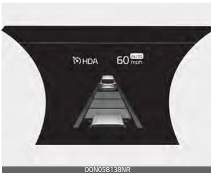
If Highway Driving Assist operating conditions are all met and setting speed matches with the legal high-
