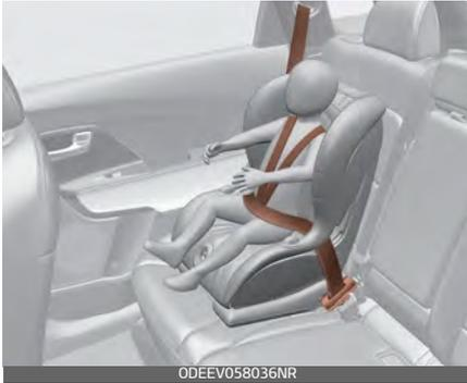
A forward-facing child seat provides restraint for the child's body with a harness. Keep children in a forward-facing child seat with a harness until they reach the top height or weight limit allowed by your child restraint's manufacturer. Once your child outgrows the forward-facing child restraint, your child is ready for a booster seat.
