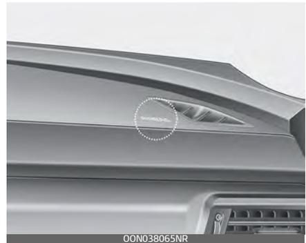
The indication of the system's presence are the letters "AIR BAG" located on the air bag pad cover on the steering wheel and the passenger's side front panel pad above the glove box.
