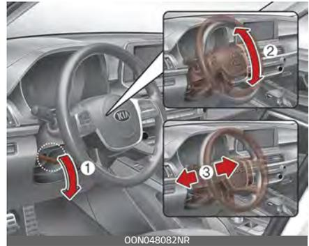
1. To change the steering wheel angle, pull down the lock release lever (1).
