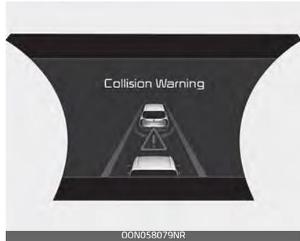
The warning message appears on the LCD display with a warning chime.
