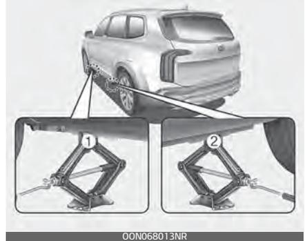
8. Insert the wheel lug nut wrench into the jack and turn it clockwise, raising the vehicle until the tire just clears the ground. This measurement is approximately 1 in (30 mm).
