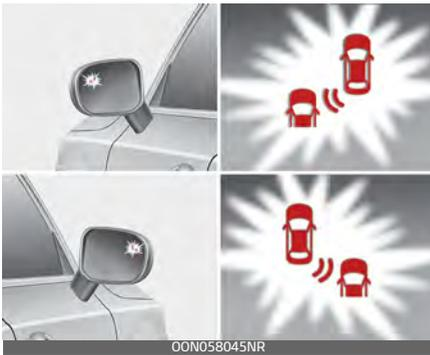
If a vehicle is detected within the boundary of Blind-Spot Collision Warning, a warning light will illuminate on the outside rearview mirror and the Head-Up Display (if equipped).
