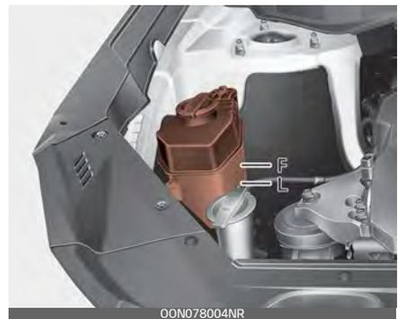
Do not remove the radiator cap when the engine and radiator are hot. Scalding hot coolant and steam
