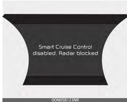
When the sensor lens cover is covered with dirt, snow, or debris, Smart Cruise Control operation may stop temporarily. If this occurs, a warning message will appear on the LCD display. Remove any dirt, snow, or debris and clean the radar sensor lens cover before operating Smart Cruise Control.
