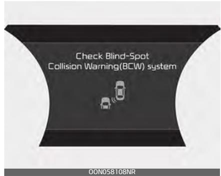
If there is a problem with Blind-Spot Collision Warning, a warning message will appear and the light on the switch will turn off. Rear Cross-Traffic Collision Warning and Rear Cross-Traffic Collision-Avoidance Assist will turn off automatically. Rear Cross-Traffic Collision Warning and Rear Cross-Traffic Collision-Avoidance Assist will not operate also if Blind-Spot Collision Warning turns off due to malfunction. Have your vehicle inspected by an authorized Kia dealer.
