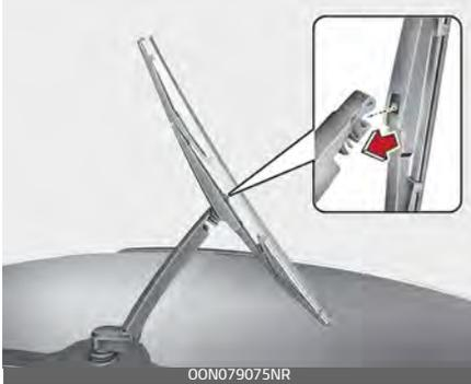
3. Make sure the blade assembly is installed firmly by trying to pull it slightly.
