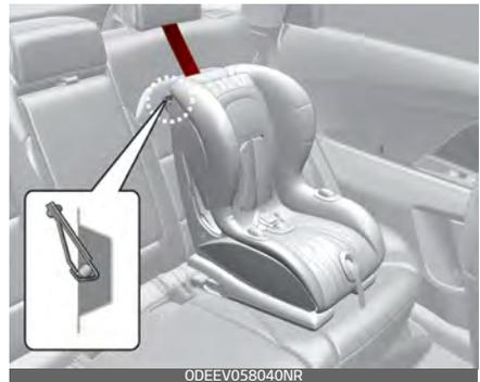
1. Route the child restraint tether strap over the child restraint seatback. Route the tether strap
