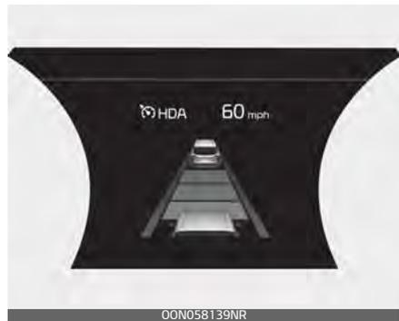
If the driver directly changes the speed, it enters the manual speed setting mode and the set speed is displayed in white and the "AUTO" symbol will disappear.
