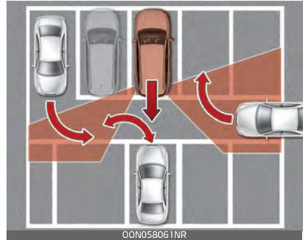
Rear Cross-Traffic Collision Warning and Rear Cross-Traffic Collision-Avoidance Assist may not operate properly when the vehicle is in a complex parking environment.
