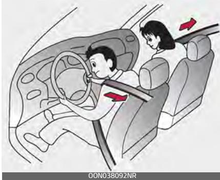
Your vehicle is equipped with pre-tensioner seat belts at the front outboard seating positions.
