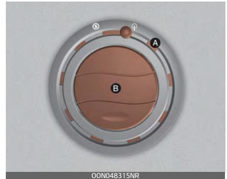
: Air discharged from [A] spreads over a wider area.
