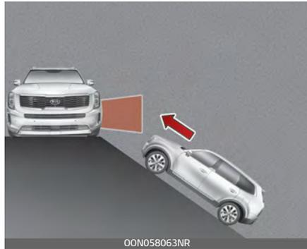
Rear Cross-Traffic Collision Warning and Rear Cross-Traffic Collision-Avoidance Assist may not operate properly when the vehicle is on/near a slope.
