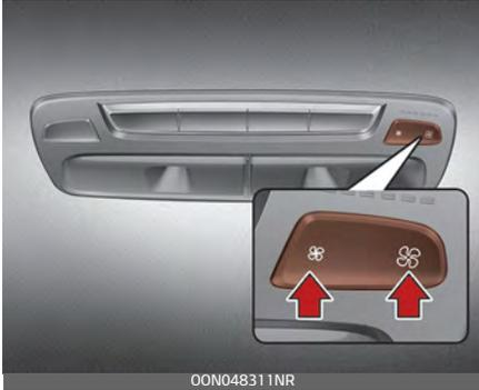
1. To change the rear fan speed, press the button (⊕) for higher speed, or press the button (⊖) for lower speed.
