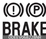
Check the brake warning light by turning the ENGINE START/STOP button ON (do not start the engine). This light will be illuminated when the parking brake is applied with the ENGINE START/STOP button in the START or ON position.
