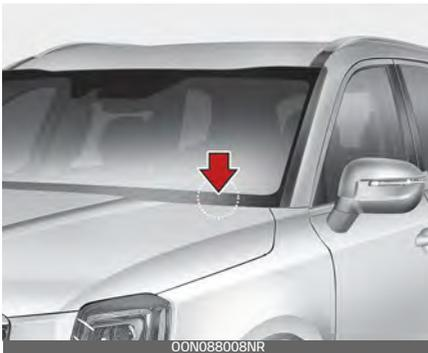
The VIN is also on a plate attached to the top of the dashboard. The number on the plate can easily be
