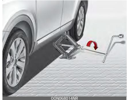
Before removing the wheel lug nuts, make sure the vehicle is stable and that there is no chance for movement or slippage.
