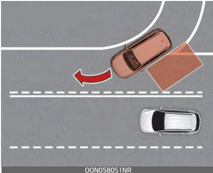
Blind-Spot Collision Warning and Blind-Spot Collision-Avoidance Assist may not operate properly when driving where the road is merging/dividing. In certain instances Blind-Spot Collision Warning and Blind-Spot Collision-Avoidance Assist may not detect the vehicle in the next lane. Always pay attention to road and driving conditions, while driving.
