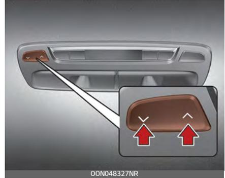
2. To change the temperature, press the button (∧) for warmer air or press the button (∨) for cooler air.
