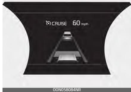
Your vehicle speed will slow down or speed up to maintain the selected distance. (A vehicle will appear in front of your vehicle in the LCD display only when there is an actual vehicle in front of you.)
