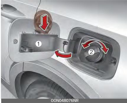
4. To remove the fuel tank cap (2), turn it counterclockwise. You may hear a hissing noise as the pressure inside the tank equalizes.
