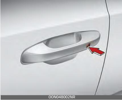
Pressing the button of the front outside door handles with all doors (and liftgate) closed and any door unlocked, locks all the doors (and liftgate).
