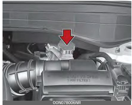
1. Before removing the reservoir cap and adding brake fluid, clean the area around the reservoir cap thoroughly to prevent brake fluid contamination.
