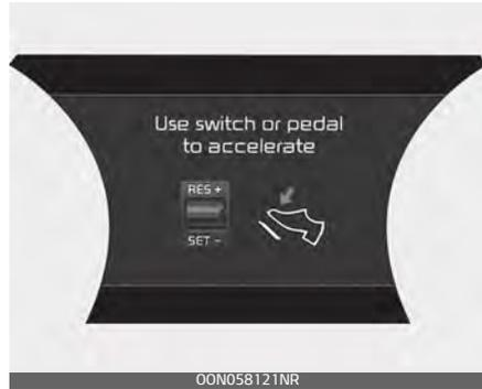
While Smart Cruise Control is in operation, your vehicle stops behind the vehicle in front when it stops. The message is displayed on the cluster within 3 seconds after the stop and the system will be in the standby position.
