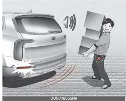
The hazard warning lights will blink and chime will sound 2 times and then the liftgate will open. Make sure you close the liftgate before driving your vehicle. Make sure there are no people or objects around the liftgate before opening or closing the liftgate. Make sure objects in the liftgate do not come out when opening the liftgate on a slope. It may cause serious
