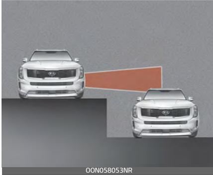
Blind-Spot Collision Warning and Blind-Spot Collision-Avoidance Assist may not operate properly when driving where the heights of the lanes are different.
