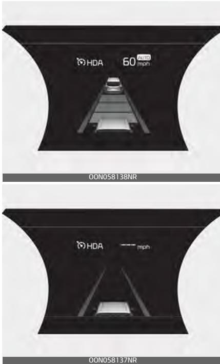
If both lanes are recognized properly (lane color: white), the steering wheel indicator (🚘) lights up in green and then the steering control is initiated. When the system cannot provide temporary steering inputs, the indicator flashes green and then changes to white. Even when the Highway Driving Assist function cannot provide temporary steering inputs, it still controls the distance from other vehicles. (For information on non-operating conditions of steering wheel control, please refer
