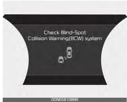
If there is a problem with Blind-Spot Collision Warning, a warning message will appear and the light on the switch will turn off. Blind-Spot Collision Warning will turn off automatically. Blind-Spot Collision-Avoidance Assist will not operate also if Blind-Spot Collision Warning turns off due to malfunction. In this case, have your vehicle inspected by an authorized Kia dealer.
