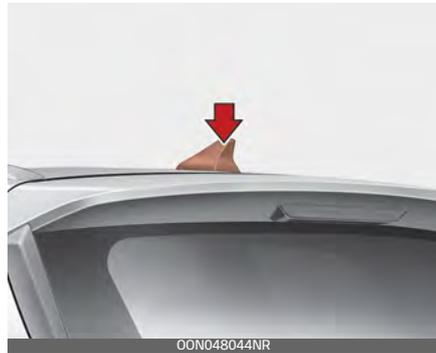
The shark fin antenna will receive the transmitted data.
