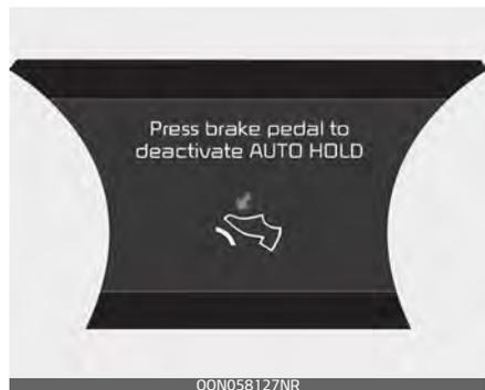
When you press the [AUTO HOLD] switch, if the driver's door and engine hood are not closed or the liftgate is not closed, a warning will
