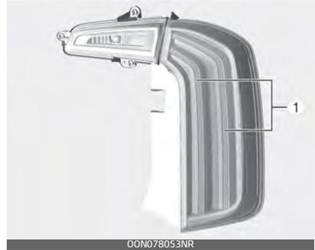
If the Stop and tail lamp (LED Type) does not operate, have your vehicle checked by an authorized Kia dealer.
