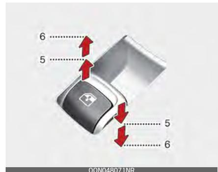
Pressing or pulling up the power window switch momentarily to the second detent position (6) completely lowers or raises the window even when the switch is released. To
