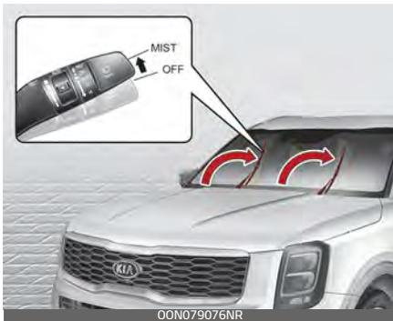
To inspect or replace the windshield wiper blades and to prevent damaging the hood, move the windshield wiper blades to the service position as follows;
