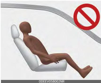
The driver must advise the passengers to keep the seatback in an upright position whenever the vehicle is in motion. If a seat is reclined during an accident, the restraint system's ability to restrain will be greatly reduced.
