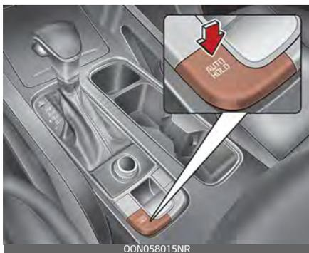
Before the Auto Hold will engage, the driver's door and engine hood must be closed and the liftgate must be closed.
