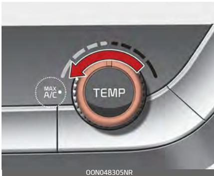
In this mode, the air conditioning and the recirculated air position will be selected automatically.
