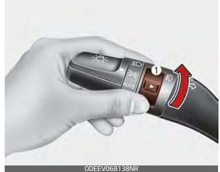
The fog lights will turn on when the fog light switch (1) is turned to the ON position after the headlight is turned on.
