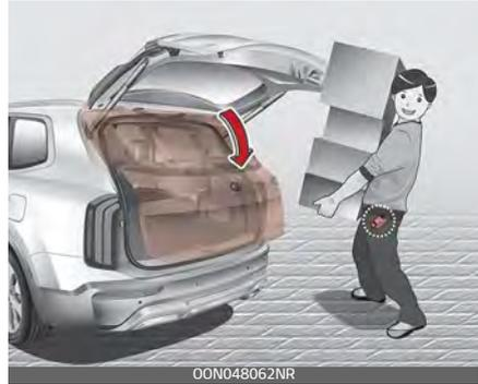
On a vehicle equipped with a smart key, the liftgate can be opened using the Smart Power Liftgate system.
