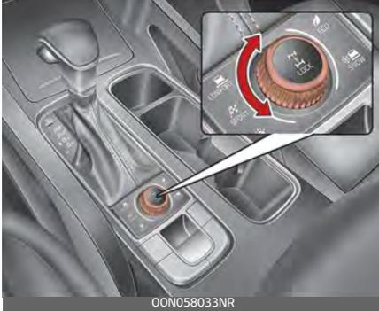
The Drive mode is activated by turning the knob.
