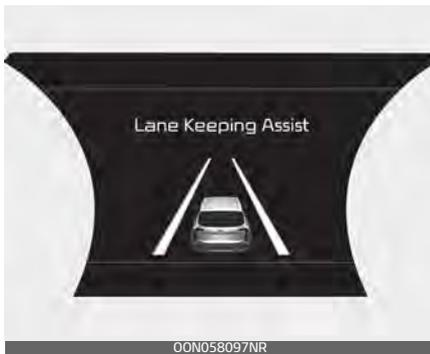
To see the Lane Keeping Assist screen on the LCD display in the cluster, Tab to the ASSIST mode (
