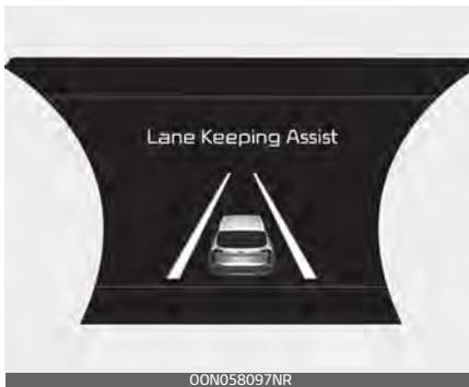
To see the Lane Keeping Assist screen on the LCD display in the cluster, Tab to the ASSIST mode (
