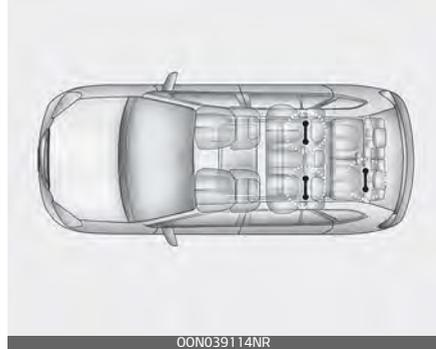
LATCH anchors have been provided in the left and right outboard of 2nd row and the left outboard of 3rd row seating positions. Their locations are shown in the illustration.
