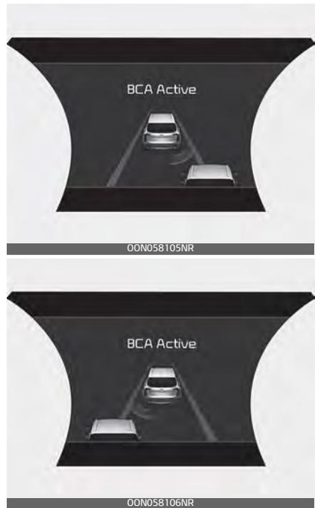
Blind-Spot Collision-Avoidance Assist may apply braking power, when an approaching vehicle is detected within a certain distance next to/behind your vehicle.
