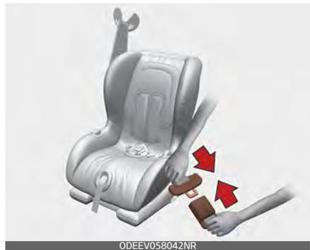
3. Pull the shoulder portion of the seat belt all the way out. When the shoulder portion of the seat belt is fully extended, it will shift
