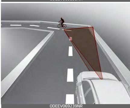
detect the vehicle, pedestrian or cyclist traveling in front on a curved road.
