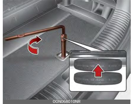
1. Place the wheel under the vehicle and install the retainer through the wheel center.
