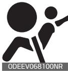
If the air bag warning light is illuminated for more than 6 seconds after the ENGINE START/STOP button has been turned to the ON position, or of it illuminates during vehicle operation, an SRS component may not be functioning properly and you should have your vehicle checked by an authorized Kia dealer.
