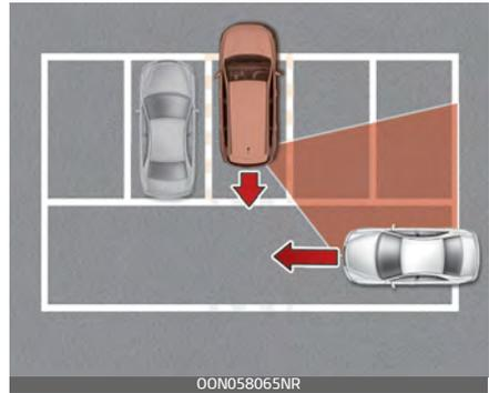
If the vehicle is parked rearward and the sensor detects the another vehicle in the rear area of the parking space, the system can warn or control braking.
