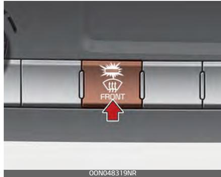
Most of the air flow is directed to the windshield with a small amount of air directed to the side window defrosters.
