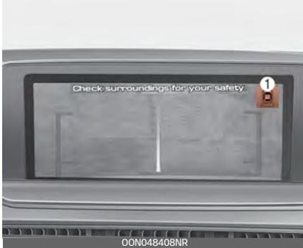
When you touch the icon (1), the top view is displayed on the screen and shows the distance from the vehicle in the back of your vehicle. Touch the icon (1) again, to switch back to the previous screen.
