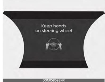
The hands-off warning appears when the system detects that the driver's hands are not on the steering wheel while Highway Driving Assist is in work. (First warning: warning message, Second warning: warning message with warning sound)
