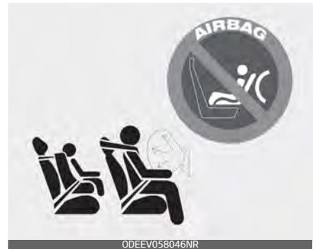
If the air bag deploys, it would impact the rear-facing child restraint, causing serious or fatal injury.
