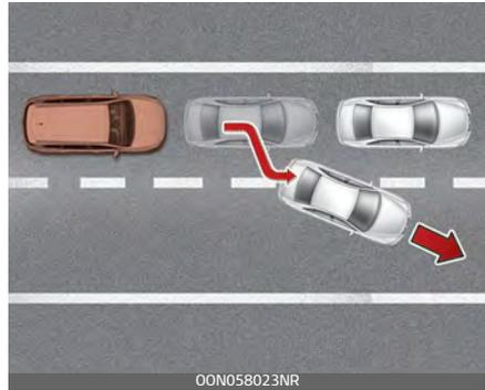
When driving in stop-and-go traffic, and a stopped vehicle in front of you merges out of the lane, Forward Collision-Avoidance Assist may not immediately detect the new vehicle that is now in front of you. In this case, you must maintain a safe braking distance, and if necessary, depress the brake pedal to reduce your driving speed in order to maintain a safe distance.
