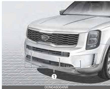
The sensing range and objects detectable by the ultrasonic sensors (1) are limited. Whenever moving
