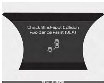
If there is a problem with Blind-Spot Collision-Avoidance Assist, a warning message will appear. Blind-Spot Collision-Avoidance Assist will turn off automatically. Blind-Spot Collision Warning will still operate even if Blind-Spot Collision-Avoidance Assist turns off due to malfunction. In this case, have your vehicle inspected by an authorized Kia dealer.
