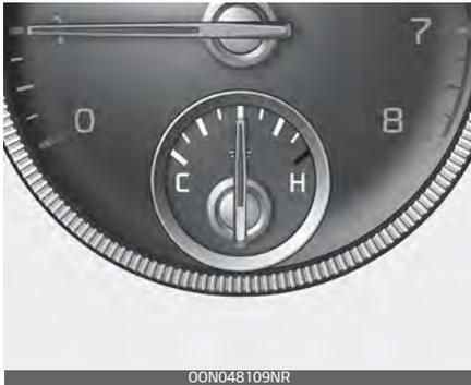
This gauge indicates the temperature of the engine coolant when the ENGINE START/STOP button or ENGINE START/STOP button is ON.
