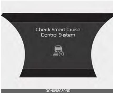
The message will appear when the vehicle to vehicle distance control system is not functioning normally.
