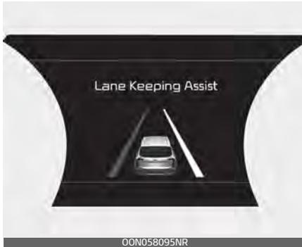
If the vehicle moves out its lane because steering torque for assistance is not enough, the line indicator of deviation direction will blink and the warning sound is provided.
