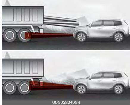
Always be cautious when approaching vehicles that are taller with higher clearance, or vehicles carrying loads that stick out of the back of the vehicle.
