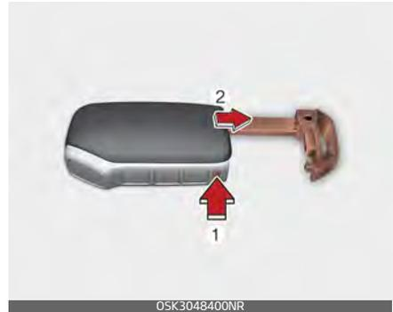
To reinstall the mechanical key, put the key into the hole and push it until a click sound is heard.
