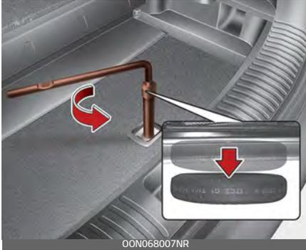
4. After the spare tire reaches the ground, continue to turn the tool counterclockwise, and draw the spare tire outside. Never rotate the tool excessively, otherwise the spare tire carrier may be damaged.
