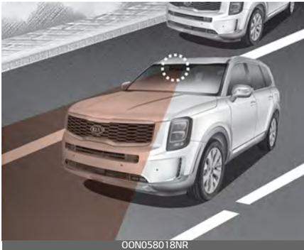
When the Lane Keeping Assist function detects the vehicle straying from its lane, it alerts the driver with a visual and audible warning, while applying a slight counter steering torque, trying to prevent the vehicle from moving out of its lane.
