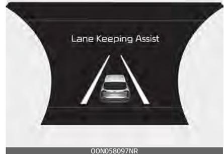
If the speed of the vehicle is over 40 mph (64 km/h) and Lane Keeping Assist detects lane markers, the color changes from gray to white.
