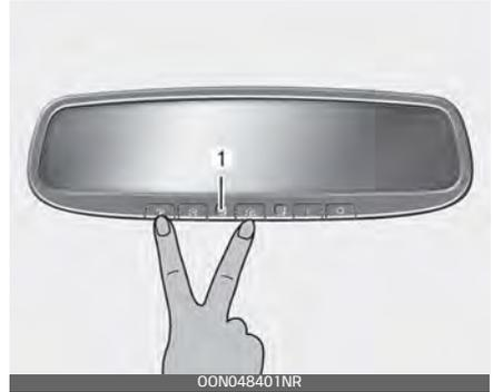
To erase the three programmed buttons (individual buttons cannot be erased):
