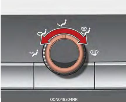
Air can be directed to the floor, dashboard outlets, or windshield. Five symbols are used to represent Face, Bi-Level, Floor, Floor-Defrost and Defrost air position.
