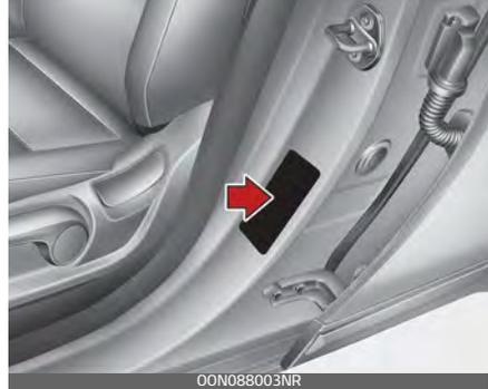
The tire label located on the driver's side center pillar gives the tire pressures recommended for your vehicle.
