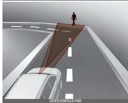
The performance of Forward Collision-Avoidance Assist may be limited when driving on a curved road.
