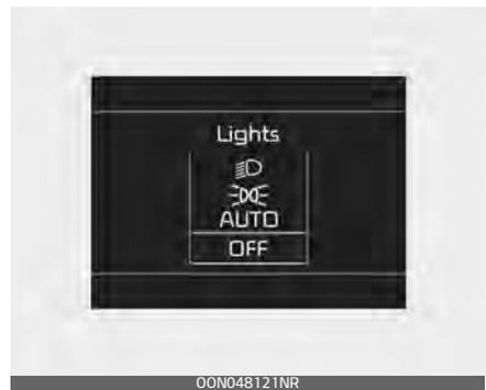
This indicator displays which exterior light is selected using the lighting control.
