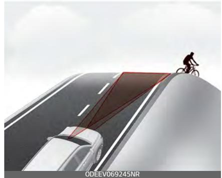
The performance of Forward Collision-Avoidance Assist may be decreased while driving upward or downward on a slope. The front view camera or front radar sensor recognition may not detect the vehicle, pedestrian or cyclist in front.
