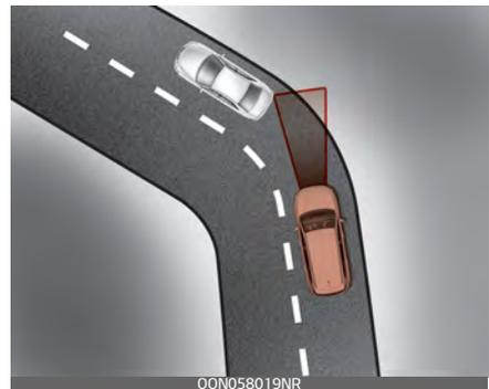
The Smart Cruise Control function may not detect a moving vehicle in
