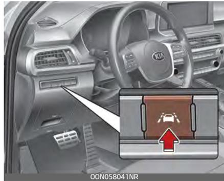
To activate and deactivate Lane Keeping Assist, with the ENGINE START/STOP button in the ON position, take the following steps:
