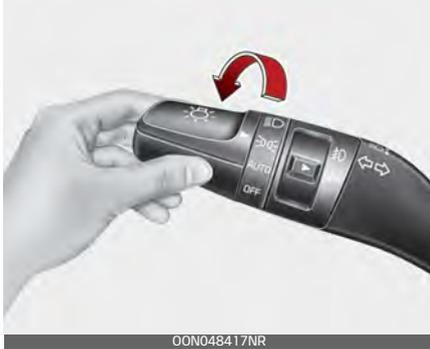
When the light switch is in the position lamp position, the tail, license and instrument panel lights will turn ON.
