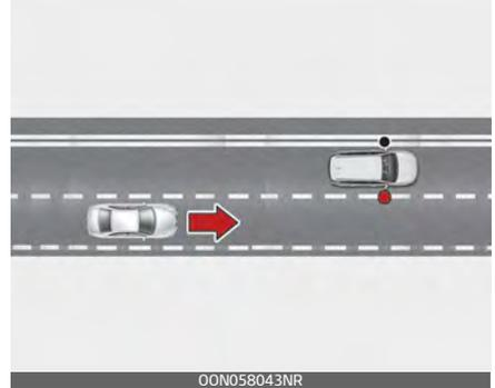
The Lane Change Assist feature will alert you when a vehicle is approaching in an adjacent lane at a high rate of speed. If the driver activates the turn signal when the system detects an oncoming vehicle, the system sounds an audible warning.
