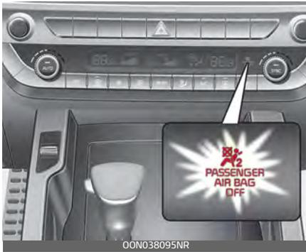
The ODS is designed to detect the presence of a properly-seated front passenger and determine if the passenger's front air bag should be enabled (may inflate) or not. Only the front passenger front air bag is controlled by the ODS.
