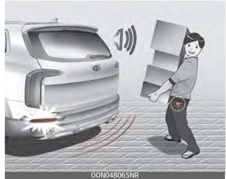
The hazard warning lights will blink and chime will sound 2 times and then the liftgate will open. Make sure you close the liftgate before driving your vehicle. Make sure there are no people or objects around the liftgate before opening or closing the liftgate. Make sure objects in the liftgate do not come out when opening the liftgate on a slope. It may cause serious
