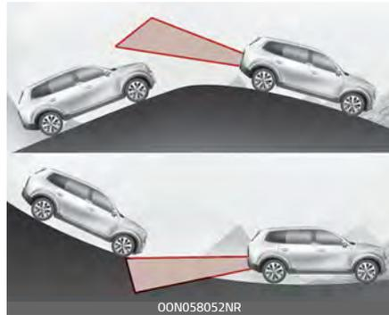
Blind-Spot Collision Warning and Blind-Spot Collision-Avoidance Assist may not operate properly when driving on a slope. In certain instances Blind-Spot Collision Warning and Blind-Spot Collision-Avoidance Assist may not detect the vehicle in the next lane.
