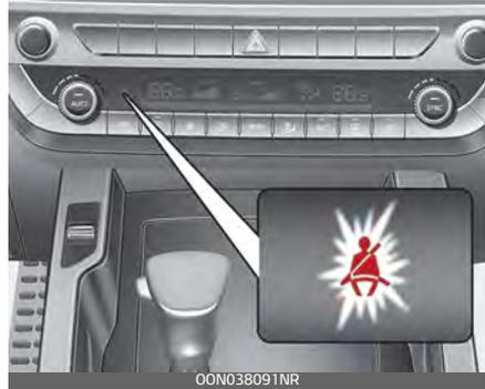
If you start to drive without the seat belt fastened or you unfasten the seat belt when you drive over 5 mph (9 km/h) and less than 12 mph (20 km/h), the corresponding warning light will illuminate. The warning light will turn off when the vehicle speed drops below 5 mph (9 km/h).
