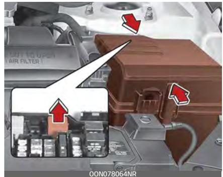
4. Check the removed fuse; replace it if it is blown. Spare fuses are provided in the engine compartment fuse panel.
