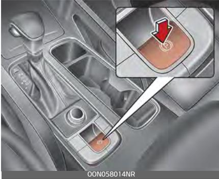
Releasing the parking brake with EPB switch,
