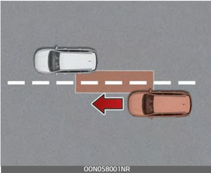
When the function detects an approaching vehicle, the rear doors will not unlock even if the driver attempts to unlock them using the electronic child safety lock button. The "Check surroundings then try again" warning message appears on the cluster and a warning sounds.
