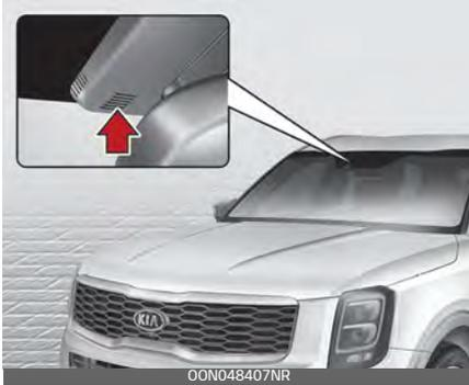
The ADS operates when the heater or air conditioning is on.
