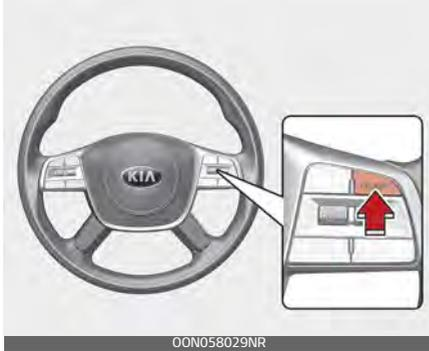
When Smart Cruise Control is not needed, press the [CRUISE] switch and deactivate the system.
