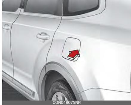
If the fuel filler door does not open because ice has formed around it, tap lightly or push on the lid to break the ice and release the lid. Do not apply excessive force to open the lid. If necessary, spray around the lid with an approved de-icer fluid (do not use radiator anti-freeze) or move the vehicle to a warm place and allow the ice to melt.
