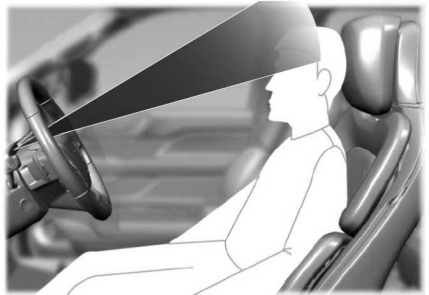
Steering column too high, camera cannot see the face.
