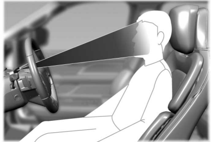
Appropriate position, camera can see the face.
