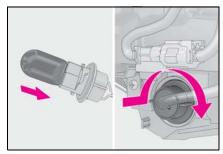
8 Align the tabs and push the light unit toward the front of the vehicle to install it.
