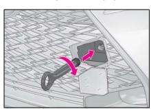
4 Tighten down the towing eyelet securely using a phillips-head screwdriver or hard metal bar.
