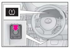
Wait for a few minutes with the engine switch in IGNITION ON mode and then turn the engine switch off.
