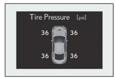
If the tire pressure drops below a predetermined level, the driver is warned by a screen display and a warning light. (->P.307)
