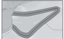
2 Using a flathead screwdriver, remove the cover.
