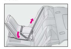
5 After installing the child restraint system, rock it back and forth to ensure that it is installed securely.
