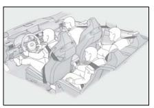
The pretensioners help the seat belts to quickly restrain the occupants by retracting the seat belts when the vehicle is subjected to certain types of severe frontal collision or a vehicle rollover.
