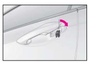
• The trunk is opened using the mechanical key.
