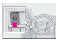
Temporarily switching to the low beams
