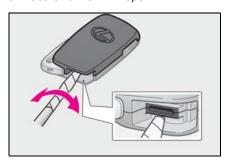
Remove the depleted battery.
