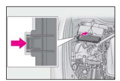
► Engine compartment: type B fuse box
