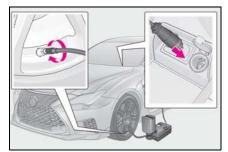
20 Turn the compressor switch on and wait for several seconds, then turn it off. Check the tire inflation pressure.
