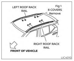
1. Manually remove all 8 protective caps from the roof rack rails. See Fig. 1.
