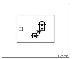
The Blind Spot Warning (BSW) switch is used to turn on and off the BSW system. When the BSW switch is pushed, the BSW system will turn on and the BSW indicator light in the meter will illuminate. When the BSW switch is pushed again, the BSW svstem will turn off and the BSW indicator light will turn off
