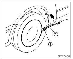
Removing wheel cover (if so equipped)
