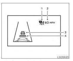
Vehicle-to-vehicle distance control mode display and indicators
