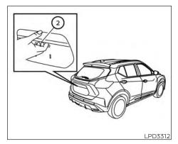
Doors do not lock with the door handle request switch (if so equipped) with the Intelligent Key inside the vehicle and a beep sounds to warn you. However, when an Intelligent Key is inside the vehicle, doors can be locked with another Intelligent Key.
