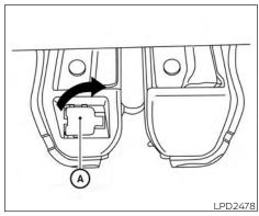
1. Move the cover (A) by using a screwdriver or a similar tool available on hand.
