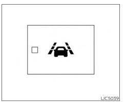
The Lane Departure Warning (LDW) switch is used to turn on and off the LDW system. When the LDW switch is pushed, the LDW system will turn on and the LDW indicator light will illuminate. When the LDW switch is pushed again, the LDW system will turn off and the LDW indicator light will turn off.
