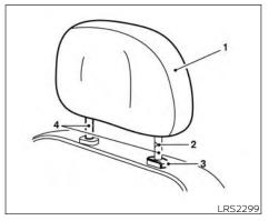
NON-ADJUSTABLE HEAD RESTRAINT/HEADREST COMPONENTS
