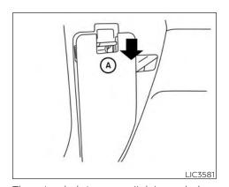
The extended storage switch is used when the vehicle is in transit from the factory. It is located in the fuse panel (A) which is on the driver's side left kick panel, near the floor, on the inside of the panel. If any electrical equipment does not operate, ensure the extended storage switch is pushed fully in place, as shown.
