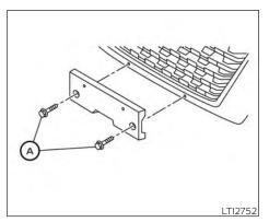
To install the front license plate bracket: Use two 6 mm screws (A) to attach front license plate bracket to radiator grille.
