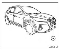
The I-FCW system can help alert the driver when there is a sudden braking of a second vehicle traveling in front of the vehicle ahead in the same lane.
