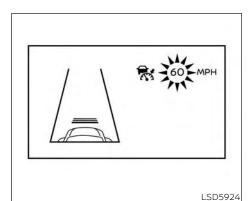
When passing another vehicle, the set speed indicator will flash when the vehicle speed exceeds the set speed. The vehicle detect indicator will turn off when the area ahead of the vehicle is open. When the pedal is released, the vehicle will return to the previously set speed.
