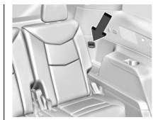
Insert the SD card into the card reader in the trim panel of the left-hand rear seat. Disable the system from the playback screen before removing the SD card from the reader. Do not remove the card while recording is enabled. This could corrupt the video file and/or the SD card.
