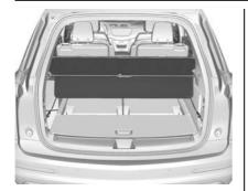
If equipped, the cargo cover is used to cover items in the cargo area. It is foldable and stores in the cargo storage bin under the load floor when not in use.
