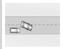
Super Cruise may not detect a vehicle that enters your lane, or may not brake fast enough to avoid a crash. You must manually brake and steer the vehicle.
