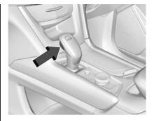
This vehicle is equipped with an electronically controlled transmission. The shift lock release button is designed to prevent inadvertent shifting out of P (Park) unless the vehicle is on, the brake pedal is applied, and the shift lock release button is pressed.
