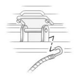
6. Open the lift gate to 3 / 4 door location and adjust the door automatically or manually until there is enough space to hook the cable to the door hinges. See Liftgate \$\phi\$ 25.
