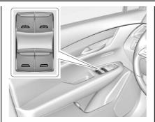
The power windows work when the ignition is on, in accessory mode, or when Retained Accessory Power (RAP) is active. See Retained
