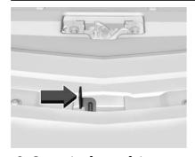
Go to the front of the vehicle and locate the secondary release lever under the front center of the hood. Push the secondary hood release lever to the right to release.  After you have partially lifted the hood, the gas strut system will automatically lift the hood and hold it in the fully open position.
