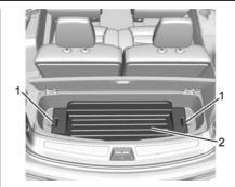
Remove the cargo management system tray (2) by pulling on the handles (1). See Cargo Management System
