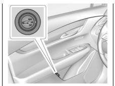
The power liftgate switch is on the driver door. The vehicle must be in P (Park).
