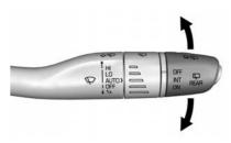
The rear window wiper/ washer controls are on the end of the windshield wiper lever. Turn the controls to adjust the setting.
