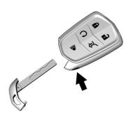
To remove the key, press the button on the side of the remote key, near the bottom, and pull the key out. Never pull the key out without pressing the button.
