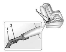
Lower anchors (1) are metal bars built into the vehicle.
