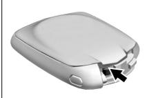
Separate the two halves of the remote key using a flat tool inserted into the bottom center of the remote key. Do not use the key slot.
