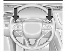
If equipped, vehicles with Tap Shift have controls on the back of the steering wheel to manually shift the automatic transmission.
