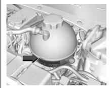
Check to see if coolant is visible in the coolant surge tank. If the coolant inside the coolant surge tank is boiling, do not do anything else until it cools down. If coolant is visible but the coolant level mark is not at or above the indicated mark, add a 50/50 mixture of clean, drinkable water and DEX-COOL coolant. Be sure
