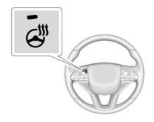
If equipped, press to turn on or off. A light near the button displays when the feature is turned on.
