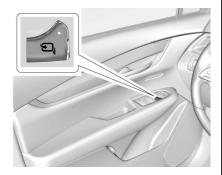
If equipped, press  $\square_i$  to power fold the mirrors. Press  $\square_i$  again to unfold.
