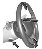
Power Tilt and Telescoping Steering Wheel
