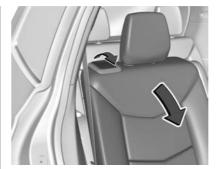
Pull the handle on the top of the seat forward and pull the seat forward.
