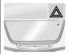
▲: Touch ▲ on the center stack to make the front and rear turn signal lamps flash on and off. Touch again to turn the flashers off.
