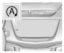
The automatic engine Stop/ Start feature can be disabled and enabled by touching the (A) symbol. Auto Stop is enabled each time you start the vehicle. When the light next to the (A) is illuminated, the system is enabled.
