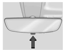
Pull the tab to turn on the display. Push the tab to turn it off. When off the mirror is
