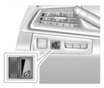
This feature adjusts the brightness of all illuminated controls. This feature is on the left side of the instrument panel.
