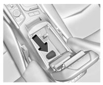
3. Place the new remote key into the remote key pocket. The remote key pocket is inside the center console storage area between the driver and front passenger seats. The storage area will need to be opened and the storage tray lifted up to access the remote key pocket.
