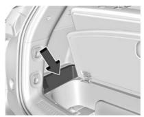
The rear compartment fuse block is in the cargo area, on the driver side of the vehicle behind the lower trim panel. To access the fuses in the Rear Electrical Center, remove the center cargo bin, then small side bin. See Rear Storage \$109. See your dealer if additional assistance is needed.
