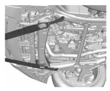
The vehicle is equipped with specific attachment points to be used by the towing provider. These holes may be used to pull the vehicle from a flat road surface onto the flatbed tow truck.
