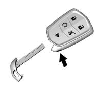
Press the button on the side of the remote key near the bottom and pull the key out. Never pull the key out without pressing the button.
