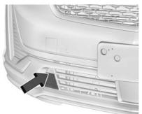
2. Remove the engine heater connector cover by gently prying with a flat-bladed tool at the location of the notch along the top edge of the cover.
