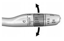
AUTO: If equipped with Rainsense, use this setting for intermittent wipes when Rainsense is disabled, or Rainsense wipes when Rainsense is enabled. For intermittent wipes, move the windshield wiper lever to AUTO, then turn the band up for more frequent wipes or down for less frequent wipes. If Rainsense is turned on, see "Rainsense" later in this section.
