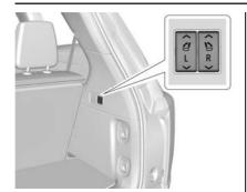
2. To return the seatback to the seating position from the cargo area, press and hold the seatback folding switch on the passenger side of the rear cargo area.
