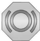
The brake/hydraulic clutch fluid reservoir cap has this symbol on it. See *Engine Compartment Overview* ⇨ 224 for reservoir location. The common hydraulic clutch and brake master cylinder fluid reservoir is filled with brake fluid as indicated on the reservoir cap. See *Brake Fluid* ⇨ 244 for brake fluid to use.
