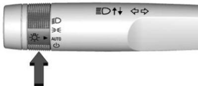
The exterior lamp control is on the left side of the steering wheel.
