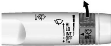
**INT** : Move the lever up to INT for intermittent wipes, then turn the
