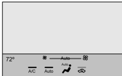
The climate control status display appears briefly when the climate controls on the center stack are adjusted.
