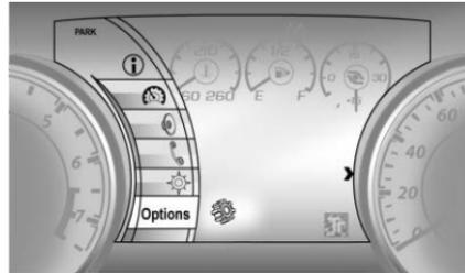
1. Using the buttons on the right side of the steering wheel, press  $\triangleleft$  to open the top level DIC menu. Use  $\nabla$  to scroll down to Options and press SEL.
