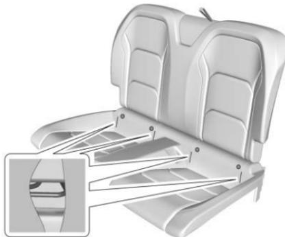
The outboard lower anchors are behind the vertical openings in the seat trim.
