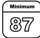
Use regular unleaded gasoline meeting ASTM specification D4814 with a posted octane rating of 87 — (R+M)/2 — or higher. Do not use gasoline with a posted octane rating of less than 87, as this may cause engine knock and will lower fuel economy.
