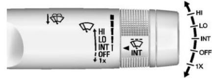
The windshield wiper/washer lever is on the right side of the steering column. With the ignition on or in ACC/ACCESSORY, move the windshield wiper lever to select the wiper speed.
