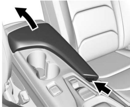
Press to open. There are two USB ports and an auxiliary jack inside. See the infotainment manual.
