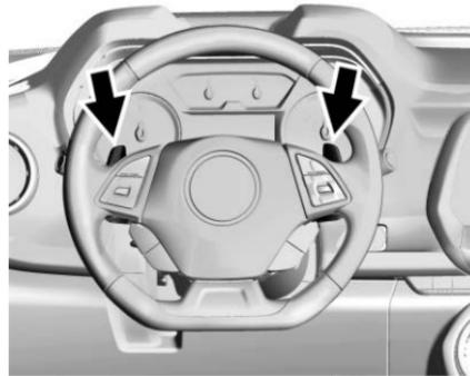
Tap Shift allows you to manually control the automatic transmission. To use Tap Shift, the shift lever must be in DSC mode. Vehicles with this feature have indicators on the steering wheel. The paddles are on the back of the steering wheel. Tap the left paddle (-) to downshift, and the right paddle (+) to upshift. The
