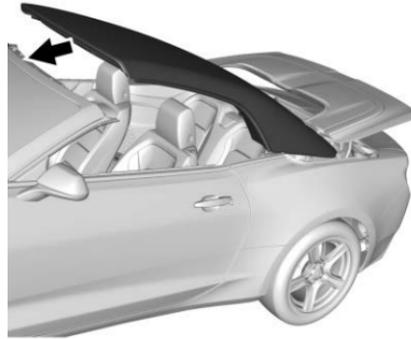
2. Lift and move the convertible top forward by pulling on both sides of the front bow into the fully closed position.
