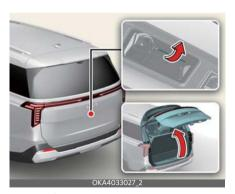
The liftgate is locked or unlocked when all doors are locked or unlocked with the transmitter (or smart key) or central door lock switch.
