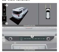
3D view function shows the vehicle in various angles. Press the 3D view icon on the Surround View Monitor screen to choose the angle. Press the 3D view icon again to reset the angle.
