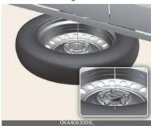
Place the wheel under the vehicle and install the retainer (1) through the wheel center. 3. Turn the wrench clockwise until it clicks.
