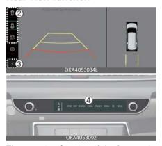
The rear-view function of the Surround View Monitor displays the vehicle's rear situation on the navigation system according to the driver's settings, assisting in safe parking.
