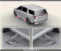
8. Insert the wheel lug nut wrench into the jack and turn it clockwise, raising the vehicle until the tire just clears the ground. This measurement is approximately 30 mm (1.2 in). Before removing the wheel lug nuts, make sure the vehicle is stable and that there is no chance for movement or slippage.
