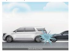
Front airbags may not inflate in side impact collisions, because passengers move in the direction of the collision. Thus, in side impacts, frontal airbag deployment would not provide additional occupant protection.
