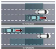
Blind-Spot Collision-Avoidance Assist can help detect and informs the driver that a vehicle is approaching at high speed from the blind spot area.
