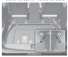
4. Tighten the fixing belt securely.
