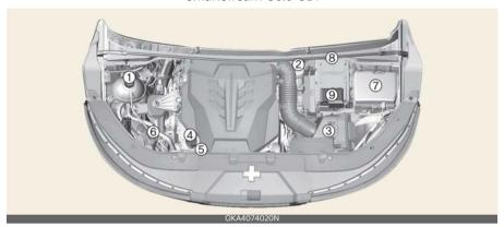
\* The actual engine compartment in your Kia may differ from the illustration. 1. Engine coolant reservoir 8-16 2. Brake fluid reservoir 8-19 3. Air cleaner 8-20 4. Engine oil filler cap 8-14 5. Engine oil dipstick 8-14 6. Windshield washer fluid reservoir 8-20 7. Fuse box 8-45 8. Negative battery terminal 7-4, 8-26
