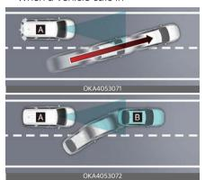
[A]: Your vehicle, [B]: Front vehicle If a vehicle cuts in front of you, Leading Departure Alert may not operate properly.
