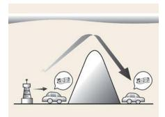
AM broadcasts can be received at greater distances than FM broadcasts. This is because AM radio waves are transmitted at low frequencies. These long distance, low frequency radio waves can follow the curvature of the earth rather than traveling straight. In addition, they curve around obstructions
