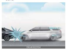
Front air bags are not designed to inflate in rear collisions, because occupants are moved backward by the force of the impact. In this case, inflated air bags would not be able to provide any additional benefit.
