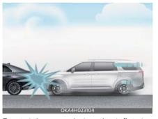
Front air bags are designed to inflate in a frontal collision depending on several factors, including the severity of impact of the front collision.
