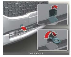
Install the towing hook by turning it clockwise into the hole until it is fully secured. 4. Remove the towing hook and install the cover after use.
