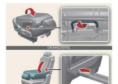
Pull the removal strap or lever and lift the rear portion of the seat cushion. Then the rear catches will be released. Remove the seat while lifting up the rear portion of seat cushion and then reinstalling the tumble seat.
