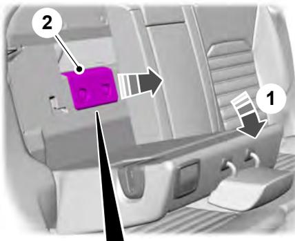
4. Slide the handle on the service disconnect outboard to the right. For Energi vehicles slide the handle outboard and to the left.
