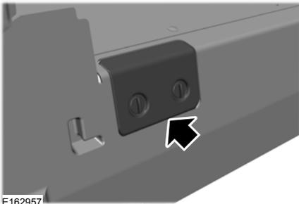
3. Pull the outer cover off to expose the service disconnect lever.
