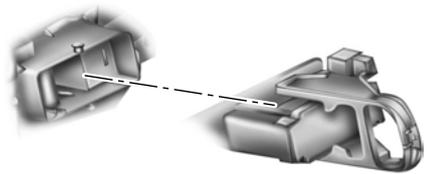
5. Pull the handle toward you and remove the circuit from the vehicle to disable the high-voltage battery.
