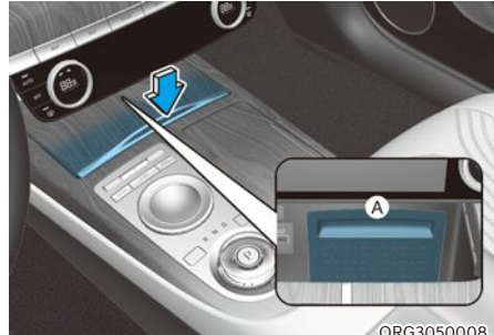
[A] : In-vehicle authentication pad (Wireless charging pad)
