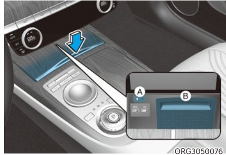
[A] : Indicator light, [B] : Charging pad
