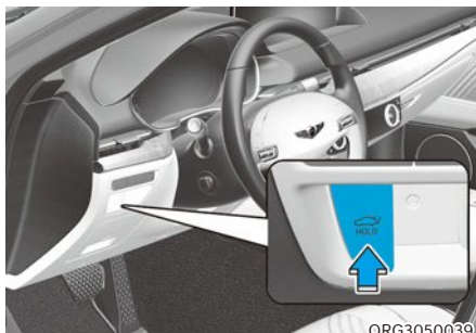
1. Power Trunk Main Control button
