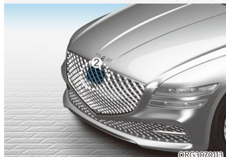
[1]: Front view camera, [2]: Front radar
