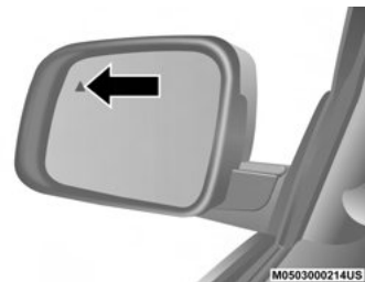
Warning Light Location
