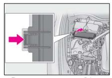
▶ Engine compartment: type B fuse
