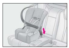
4 Fully extend the shoulder belt and allow it to retract to put it in lock
