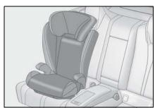
Sit the child in the child restraint system. Fit the seat belt to the child restraint system according to the manufacturer's instructions and insert the plate into the buckle. Make sure that the belt is not
