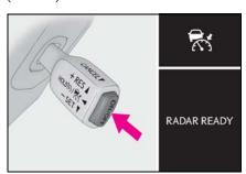
Accelerate or decelerate, with accelerator pedal operation, to the desired vehicle speed (at or above approximately 30 mph [50 km/h]) and push the lever down to set the speed.
