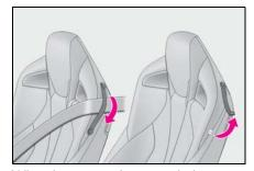
When fastening a front seat belt, ensure that it is passed through the seat belt guide. Passing the seat belt through the guide enables the seat belt to be easily extended.
