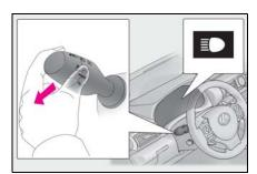
2 Press the Automatic High Beam switch.
