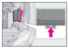
Driver's side instrument panel Remove the lid.
