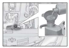
Start the engine and turn the air conditioning system on to check that the radiator cooling fans operate and to check for coolant leaks from the radiator or hoses.
