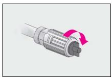
If the air release cap is not attached, the sealant may leak and the vehicle may get dirty.
