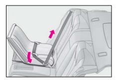
5 After installing the child restraint system, rock it back and forth to ensure that it is installed securely. (→P.49)
