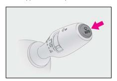
Operation of the intermittent windshield wipers with interval adjuster
