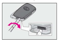
3 Remove the depleted battery.
