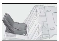
2 Run the seat belt through the child restraint system and insert the plate
