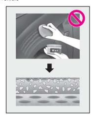
Do not wax the vehicle or apply a coating to the vehicle body, as they will form a film over the painted surfaces, filling the matte clear coat surface, making it more flat. As a result, it will become more glossy, possibly permanently losing its matte properties.
