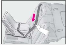
4 While pushing the child restraint system down into the rear seat, allow the shoulder belt to retract until the child restraint system is securely in place.
