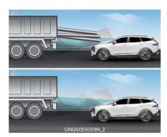
In the following cases, the vehicle in front cannot be detected by the sensor. Always pay attention to the road and driving conditions and drive safely. If necessary, adjust your vehicle speed.
