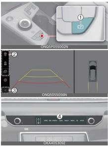
The rear view function of the Surround View Monitor displays the vehicle's rear situation on the navigation system according to the driver's settings, assisting in safe parking.
