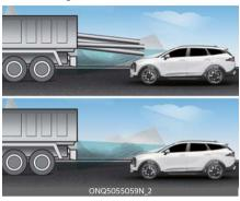
If the vehicle in front of you has cargo that extends rearward from the cab, or when the vehicle in front of you has higher ground clearance, additional special attention is required. Forward Collision-Avoidance Assist may not be able to detect the cargo extending from the vehicle. In these instances, you must maintain a safe braking distance from the rearmost object, and if necessary, steer your vehicle and depress the brake pedal to reduce your driving speed in order to maintain distance.
