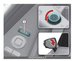
The position of the outside rearview mirror switch (1) determines whether the mirrors will move:
