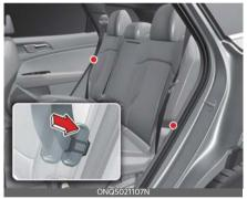
4. Pull on the seatback folding lever, then fold the seat toward the front of the vehicle. When you return the seatback to its upright position, always be sure it has locked into position by pushing on the top of the seatback.
