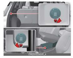
The devices should draw less than 15 amps with the vehicle on.
