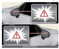
The warning light on the cluster, outside rear view mirror (side view mirror) and head-up display (if equipped) will appear when the vehicle on both lanes is detected from the rear.
