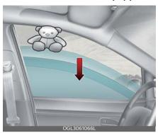
If the upward movement of the window is blocked by an object or part of the body, the window will detect the resistance and will stop upward movement. The window will then lower approximately 30 cm (12 inches) to allow the object to be cleared.
