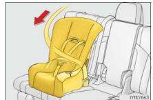
While pushing the child restraint system into the second seat or the third outboard seat (if equipped), allow the shoulder belt to retract until the child restraint system is securely in place.
