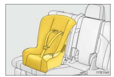
A Run the seat belt through the child restraint system and insert the plate into the buckle. Make sure that the belt is not twisted.
