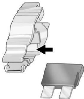
3. Use the fuse puller to remove the fuse from the top or side, as shown above.
