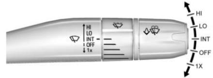
With the ignition on or in accessory mode, move the windshield wiper lever to select the wiper speed.
