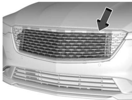
The vehicle may have a shutter system designed to help improve fuel economy. Always keep the shutter system clear of debris, snow and ice. If the check engine light is activated, please check to see if the shutter system is clear of debris, snow or ice.
