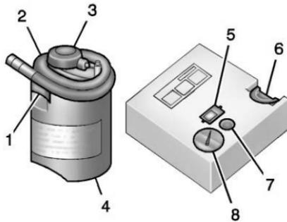
1. Sealant Canister Inlet Valve
