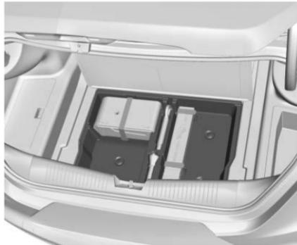
Lift up on the load floor and push forward.
