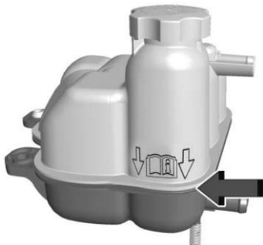
If coolant is visible but the coolant level is not at or above the indicated mark, add a 50/50 mixture of clean drinkable water and DEX-COOL coolant.
