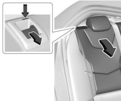
2. Pull the lever on top of the seatback toward you to unlock the seatback. A red tab near the seatback lever raises when the seatback is unlocked.
