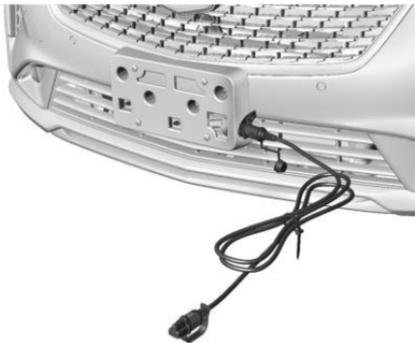
3. Plug the heater cord into the connector in the front license plate bracket.
