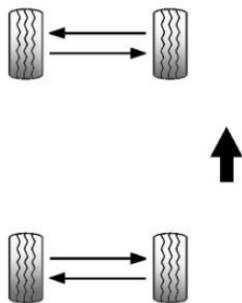
Use this rotation pattern if the vehicle has different size tires on the front and rear.
