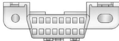
The DLC is under the instrument panel to the left of the steering wheel. Connecting devices that are not used to perform an Emissions Inspection/Maintenance test or to service the vehicle may affect vehicle operation. See *Add-On Electrical Equipment* ⇨ 285. See your dealer if assistance is needed.
