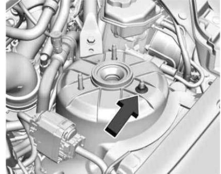
4. Loosen the final strut top mount fastener. Do not completely remove this fastener.
