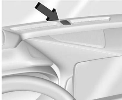
The light sensor is on top of the instrument panel or on the windshield near the rearview mirror. Do not cover the sensor, otherwise the headlamps will come on when they are not needed.
