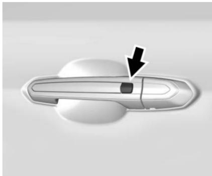
When the doors are locked and the remote key is within 1 m (3 ft) of the driver door handle, press the lock/unlock button. When unlocking from the driver door, the first press unlocks that door; press again within
