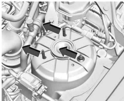
5. Reposition the suspension/strut assembly so that the strut top mount is located as close to the center of the vehicle as possible (inboard).
