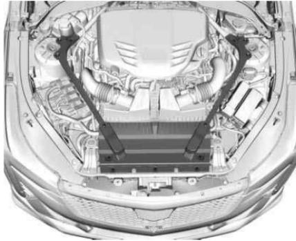
1. Remove the Upper Radiator Baffle and both front shock tower braces.
