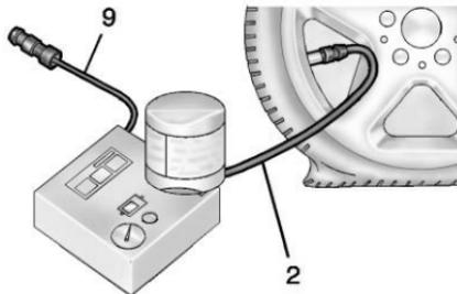
7. Attach the sealant/air hose (2) to the tire valve stem by turning it clockwise until tight.
