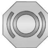
The brake/hydraulic clutch fluid reservoir cap has this symbol on it. See *Engine Compartment Overview* ⇨ 291 for reservoir location. The common hydraulic clutch and brake master cylinder fluid reservoir is filled with brake fluid as indicated on the reservoir cap. See *Brake Fluid* ⇨ 371 for brake fluid to use.
