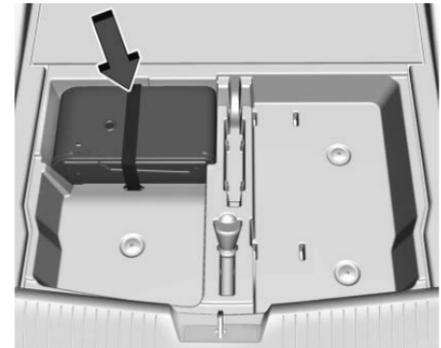
3. Remove the tire sealant and compressor kit bag.
