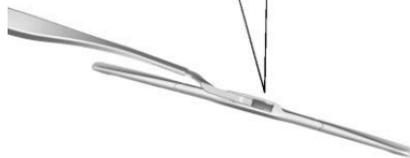
2. Lift up on the latch in the middle of the wiper blade where the wiper arm attaches.
