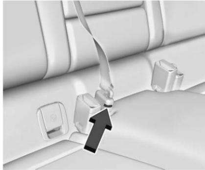
1. Disconnect the rear seat belt mini-latch using a key in the slot on the mini-buckle, and let the belt retract.
