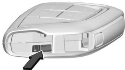
2. Use the mechanical key blade in the slot to remove the battery cover by hand.
