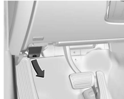
1. Pull the hood release lever with the
