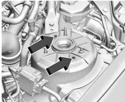
3. Using a punch, tap out the strut top mount alignment pins. Use compressed air or other method to ensure no debris remains between the top mount and upper spring seat.
