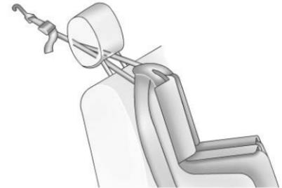
If the position you are using has an adjustable headrest or head restraint, adjust it accordingly to allow proper fitment. If you are using a dual tether, route the tether in between the headrest or head restraint posts.
