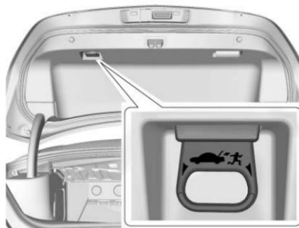
There is a glow-in-the-dark emergency trunk release handle on the trunk lid. This handle will glow following exposure to light. Pull the release handle to open the trunk from the inside.
