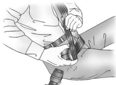
If the webbing locks in the latch plate before it reaches the buckle, tilt the latch plate flat to unlock.
