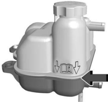
1. With a cold system, add coolant to the indicated line on the surge tank.
