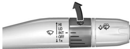
**INT** : Use this setting for intermittent wipes or for Rainsense wipes, when Rainsense is enabled. For intermittent wipes, move the lever up to INT, then turn the
