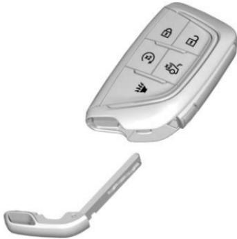
The mechanical key, inside the remote key, is used for the driver door and glove box.
