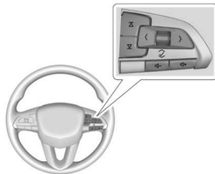
Press < or > to access the cluster applications. Use the thumbwheel to scroll ^ or v through the list of available features. Press the thumbwheel to select. Not all applications will be available on all vehicles.
