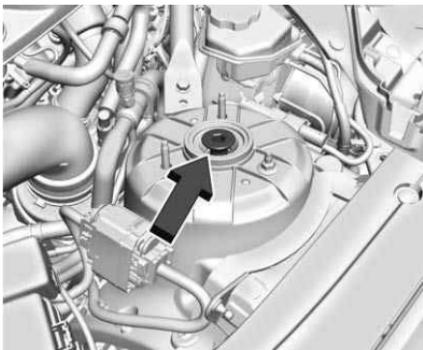
7. With the car on the ground, reinstall the strut rebound stop and torque it to 25 N•m (212 lb in).
