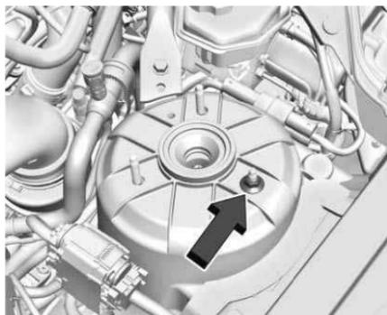
6. With the suspension located as far inboard as possible, retighten the loose fastener and torque it to 22 N•m (194 lb in).
