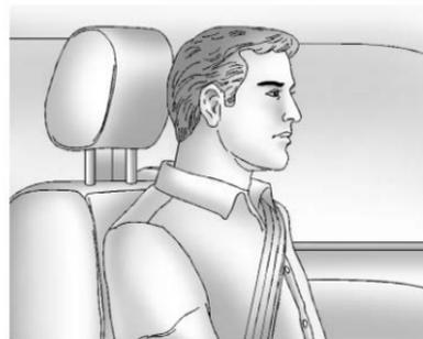
If equipped with base seats, adjust the head restraint so that the top of the restraint is at the same height as the top of the occupant's head. This position reduces the chance of a neck injury in a crash.
