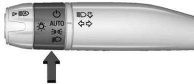
The exterior lamp control is on the turn signal lever.
