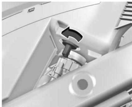
3. Turn the bulb socket counterclockwise to remove it from the headlamp assembly.
