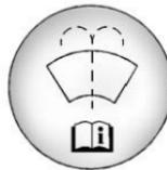
Open the cap with the washer symbol on it. Add washer fluid until the tank is full. See *Engine Compartment Overview* ⇨ 291 for reservoir location.
