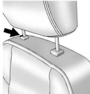
To lower the head restraint, press the button, located on the top of the seatback, and push the head restraint down. Try to move the head restraint after the button is released to make sure that it is locked in place.
