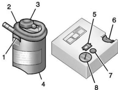
1. Sealant Canister Inlet Valve
