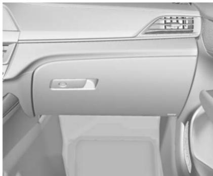
Pull the handle from the right to open the glove box. To close, push up until it latches. Use the vehicle key to lock or unlock.
