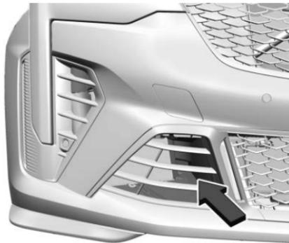
2. Front Brake Cooling Duct
