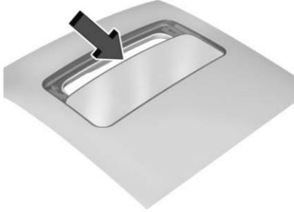
Dirt and debris may collect on the sunroof seal or in the track. This could cause an issue with sunroof operation or noise. It could also plug the water drainage system. Periodically open the sunroof and remove any obstacles or loose debris. Wipe the sunroof seal and roof sealing area using a clean cloth, mild soap, and water. Do not remove grease from the sunroof.
