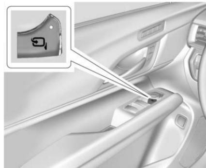
If equipped, press
