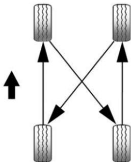
Use this rotation pattern when rotating tires of the same size installed on all four wheel positions.
