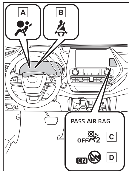
A SRS warning light
