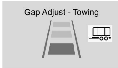
Near Gap Setting with Trailer
