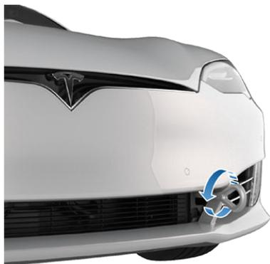
4. Attach the winch cable to the tow eye.
