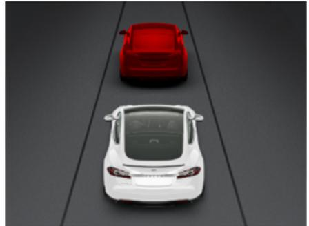
Warnings cancel automatically when the risk of a collision has been reduced (for example, you have decelerated or stopped Model S, or the object in front of your vehicle has moved out of your driving path).
