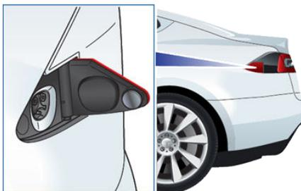
**Note:** The charge port lights up white when you open the charge port door. If you do not insert a charge cable into the charge port within a few minutes after opening the charge port door, the charge port door closes. If this happens, use the touchscreen to open the charge port door again.
