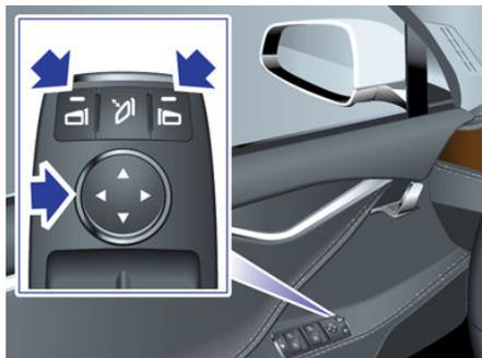
To fold and unfold exterior mirrors, press the center button. You can set the mirrors to fold automatically whenever Model S is locked by touching **Controls > Vehicle > Mirror Auto-Fold**. The mirrors unfold automatically whenever you unlock Model S.
