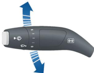
The turn signals stop operating when canceled by the steering wheel, or when you return the lever to the central position.
