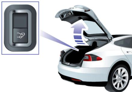
If Model S is equipped with the power liftgate, you do not need to push it up. When you press the release switch, it opens, and when you pull the switch, it closes.
