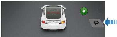
**Note:** The parking icon appears only if the vehicle's position and/or the circumstances of the surrounding area are such that Autopark can determine an appropriate driving path. If Autopark cannot determine an appropriate path (for example, when driving on a narrow street where moving into the parking space causes the front of the vehicle to extend into the adjacent lane), you can either reposition the vehicle, find a different parking space, or park manually.
