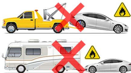
Do not transport Model S using any method that is not specified by Tesla. Adhere to the instructions provided in the following sections and observe all warnings and cautions provided. Damage caused by improper transporting of your vehicle is not covered by the warranty.
