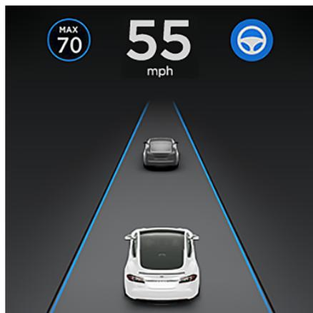
**Note:** To initiate Autosteer when there is no vehicle in front of you, you must be driving at least 18 mph (30 km/h) on a roadway with visible lane markings. If a vehicle is detected ahead of you, you can initiate Autosteer at any speed under 90 mph (150 km/h), even when stationary (if you are at least 5 feet (150 cm) away from the vehicle).
