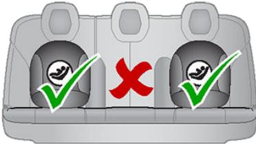
To install a LATCH child safety seat, carefully read and follow the instructions provided by the manufacturer of the child restraint system. These instructions describe how to slide the child restraint system onto the seat's anchor bars until you hear it "click" into place. You may need to push the child restraint system firmly against the seat back to ensure it fits snugly.
