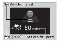
When ACC with Low Speed Follow starts operating, the vehicle icon, interval bars and set speed appear on the gauge.
