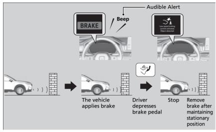
If only the rear sensors are turned off using the parking sensor system, the assistive braking will not work when reversing.
