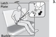
**3.** Insert the latch plate into the buckle. Properly fasten the seat belt the same way you fasten the lap/shoulder seat belt. Seat Belt with Detachable Anchor
