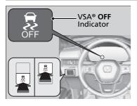
This button is on the driver side control panel. To partially disable VSA<sup>®</sup> functionality/ features, press and hold it until you hear a beep.
