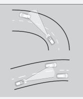
• When the vehicle ahead of you moves away, such as when entering an interchange or rest area, ACC with Low Speed Follow may continue to maintain the set following-interval for a short time.
