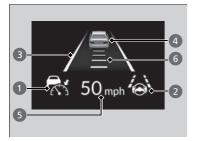
You can see the current state of Adaptive Cruise Control (ACC) with Low Speed Follow, Lane Keeping Assist System (LKAS) and Traffic Jam Assist.
