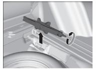
**2.** Take the tool bag out of the cargo area. Take the wheel nut wrench and jack handle bar out of the tool bag.
