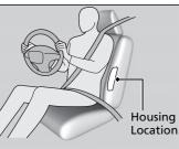
The side airbags are housed in the outside edge of the driver's, passenger's, and rear outer passenger's seat-backs.
