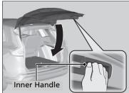
When all the doors are unlocked or you press the tailgate unlock button<sup>\*</sup> on the remote transmitter, the tailgate is unlocked. Press the tailgate outer handle and lift open the tailgate.
