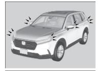
If the engine stops successfully, the exterior lights flash once.
