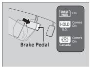
Depress the brake pedal to come to a complete stop. The transmission must not be in  $[\mathbf{P}]$  or  $[\mathbf{R}]$ .
