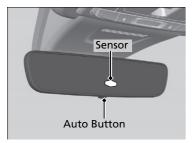
When you are driving after dark, the automatic dimming rearview mirror reduces the glare from headlights behind you. Press the AUTO button to turn this function on and off. When activated, the AUTO indicator comes on. Mutomatic Dimming Rearview Mirror\*
