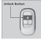
**To open:** Press the unlock button, and then within 10 seconds, press it again and hold it. If the windows stop midway, repeat the procedure.
