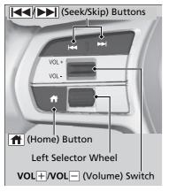
VOL //VOL (Volume) Switch Press Up: To increase the volume. Press Down: To decrease the volume. Mudio Remote Controls
