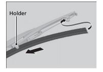
5. Slide the new wiper blade onto the holder.
