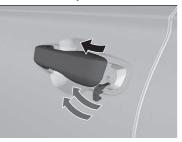
Insert the built-in key into the key cylinder from below the handle and then turn it.
