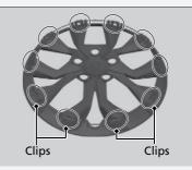
Align the valve mark on the wheel cover to the tire valve on the wheel, then install the wheel cover.
