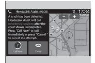
If your vehicle's airbags deploy or if the unit detects that the vehicle is severely impacted, your vehicle automatically will attempt to connect to the HondaLink operator. If connected, information about your vehicle, its location, and its condition can be sent to the operator<sup>\*1</sup>; you also can speak to the operator when connected.
