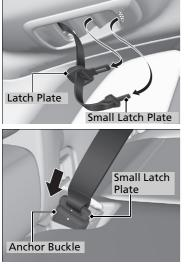
**1.** Pull out the seat belt's small latch plate and the latch plate from each holding slot in the ceiling.
