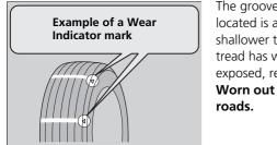
The groove where the wear indicator is located is about 1/16 inch (about 1.6 mm) shallower than elsewhere on the tire. If the tread has worn so that the indicator is exposed, replace the tire. **Worn out tires have poor traction on wet roads.**
