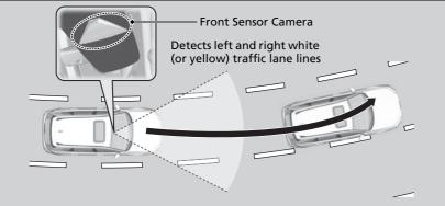
When you use the turn signal to indicate a lane change, Traffic Jam Assist is temporarily deactivated. It is reactivated once the vehicle is traveling in the center of the lane and the system has detected the traffic lane lines.
