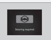
If the driver does not grip the steering wheel after the warning above has repeatedly appeared, a warning buzzer will sound and Traffic Jam Assist will be canceled.
