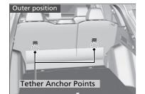
A tether anchor point is provided behind the rear outer seating positions and in the ceiling for the rear center.
