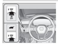
Press the heated windshield button to deice the windshield at the wiper park area and along the driver side edge of the windshield when the power mode is in ON. The heated windshield will automatically switch off after 15 minutes.
