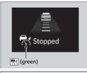
Your vehicle also stops, automatically. The **Stopped** message appears on the gauge. When the vehicle ahead of you starts again, if you press the **RES/+/SET/-** switch up or down, or depress the accelerator pedal, ACC with Low Speed Follow will operate again within the prior set speed.
