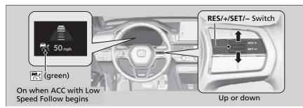
When driving at about 25 mph (40 km/h) or above: Take your foot off the pedal and press the **RES/+/SET/–** switch up or down when you reach the desired speed. The moment you release the switch, the set speed is fixed, and ACC with Low Speed Follow begins.
