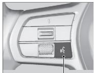
★ (Talk) button: \_\_\_\_\_ Press and hold to activate Siri. Press again to deactivate Siri. Press and release to activate standard voice recognition system.
