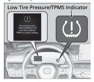
This will cause the low tire pressure/TPMS indicator to come on and a message to appear on the gauge.
