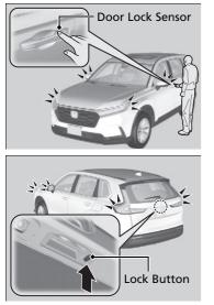
Touch the door lock sensor on the front door or press the lock button on the tailgate.
