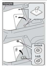
The driver's floor mat hooks over floor anchors, which keep the mat from sliding forward.
