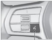
(Talk) button: \_\_\_\_\_ Press and hold to operate Android Auto with your voice. Press and release to activate standard voice recognition system. Derating Android Auto with Voice Recognition
