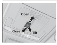
Automatic operationTo open: Pull the switch back firmly.To close: Push the switch forward firmly.
