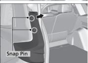
**2.** Pull the taillight carefully until the snap pins are removed from the body grommets.
