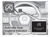
The Auto Idle Stop suspend indicator comes on and a message appears on the driver information interface when the Auto Idle Stop system cannot be activated.
