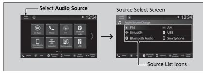
Select **Audio Source** in the header area, then select an icon on the source list to switch the audio source.
