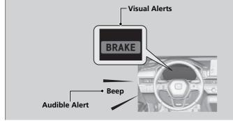
You can change the distance (**Long/Normal/Short**) between vehicles at which the system's earliest collision alert will come on.
