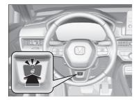
The power mode must be in ON to use the heated steering wheel.
