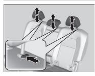
A passenger sitting in the rear seat should adjust the height of their head restraint to an appropriate position before the vehicle begins moving. **To raise the head restraint:**
