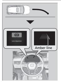
The front camera behind the rearview mirror monitors left and right lane markings in white or yellow, the outer edge of the pavement (bordered by grass or gravel) or a detected oncoming vehicles.
