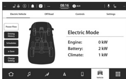
Power Flow Screen
