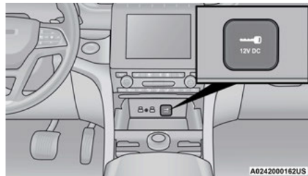
Front Power Outlet
