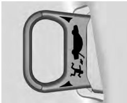
to light. Pull the release handle to open the hatch/trunk from the inside.
