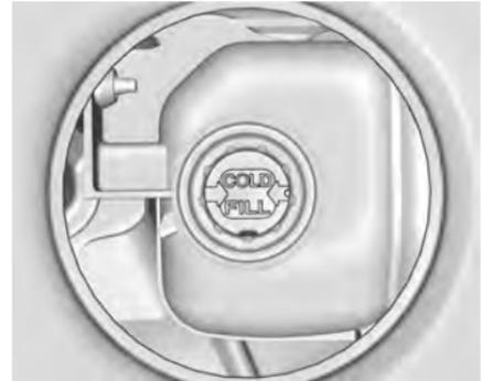
When the engine is cold, the coolant level should be at the COLD FILL indicator in the coolant surge tank.
