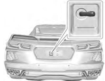
Remove the license plate to access the second backup key lock cylinder for the trunk.
