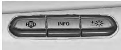
The HUD control is to the left of the steering wheel on the instrument panel.
