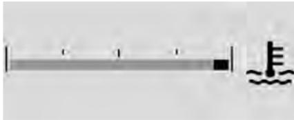
This gauge shows the engine coolant temperature.
