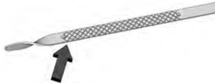
If the oil is below the cross-hatched area at the tip of the dipstick, add 1 L (1 qt) of the recommended oil through the oil fill cap opening in the oil tank fill tube and then recheck the level. See “Selecting the Right Engine Oil” later in this section for the type of oil to use. For engine oil crankcase capacity, see *Capacities and Specifications* ⇨ 300.
