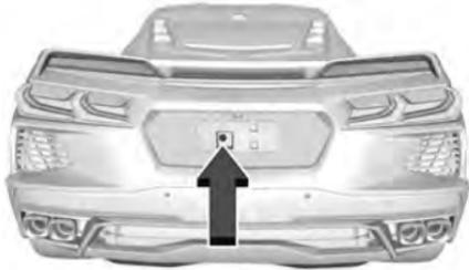
Use the mechanical key in the backup key cylinder behind the license plate to manually open the hatch/trunk. The license plate must be removed.
