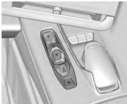
This vehicle is equipped with a dual clutch transmission that contains an integrated rear differential. The dual clutch transmission provides an extremely connected feel due to the direct connection between the engine and gear box. This arrangement provides very fast shift times for maximum performance. Automatic driving mode is selected by pulling D on the transmission range selection panel and provides fully automatic shifting operation
