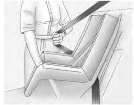
6. Pull the shoulder belt all the way out of the retractor to set the lock. When the retractor lock is set, the belt can be tightened but not pulled out of the retractor.
