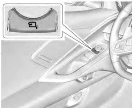
If equipped, press
