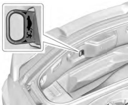
There is a glow-in-the-dark emergency hatch/trunk release handle on the inside back wall of the storage compartment. This handle will glow following exposure
