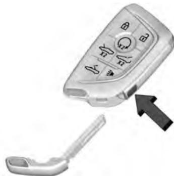
1. Press the button on the side of the remote key and pull the mechanical key out. Never pull the mechanical key out without pressing the button.
