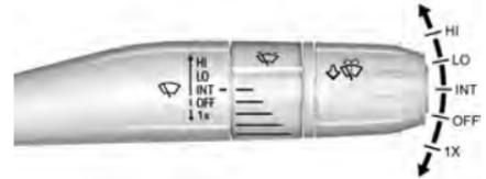
The windshield wiper/washer lever is on the right side of the steering column.
