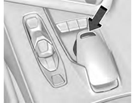
To activate My Mode, Weather, Tour, Sport and Track Mode, turn the Driver Mode Control (DMC) knob on the center console to make a mode selection. When a mode is selected, a unique and persistent indicator will be display in the driver information center (DIC).
