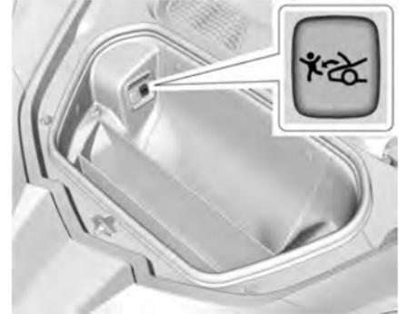
The underhood compartment is equipped with a glow-in-the-dark emergency hood release button. This button will glow following exposure to light. Press the button to open the hood from inside the underhood compartment.
