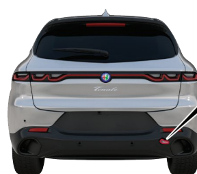
Rear Tow Eye Installed
