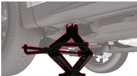
Front Jacking Location
