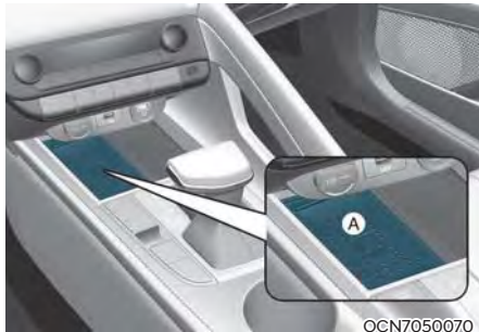
[A] : Charging pad
