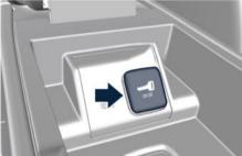
Inside the rear central tunnel compartment, under the armrest, there is a storage area for storing the key fob.
