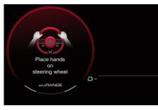
If the driver keeps his/her hands away from the steering wheel (for more than 29 seconds), also the ACC system is deactivated ( white ACC symbol on the display) and will have to be reset. In these cases the display will not show the attention level colour anymore and the vehicle will be controlled by the driver only.
