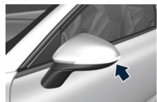
The LED turn signal indicators flash simultaneously with the corresponding turn signal lights in the front and rear of the vehicle. Turning on the hazard warning lights will also activate these LEDs.
