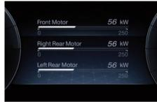
In Corsa Drive Mode, Sport bar graphs (Battery Performance or Torque) are displayed pressing and releasing the △ or ▽ button. This screen is composed by a bar graph and an instantaneous bar (vertical) on the right.
