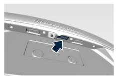
By pressing this button when the power boot lid is closed, you can open it completely, or by pressing the button again stop the opening process (after stopping, the boot lid enters in manual mode and can be only moved manually). While the boot lid is closing, by pressing this button, the boot lid can be stopped or by pressing the button again invert the movement and open it completely. When the power boot lid is open, to move it there are two buttons positioned
