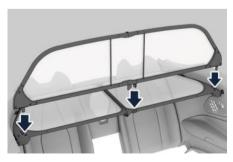
Holding the vertical element of the Windstop only by the frame, lower the center section on the horizontal element of the Windstop until both elements are engaged.
