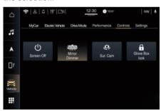
Some functions can be set only on or off touching the corresponding soft-key which will be highlighted with the yellow outline (example: "Mirror Dimmer").
