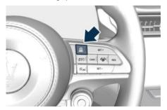
Each press and release of the button changes the time gap starting from 4 bars (default time) and moving in a
