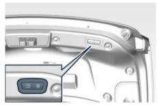
When the boot lid is completely open if you press and release the left button , the power boot lid will be completely closed unless it is stopped;
