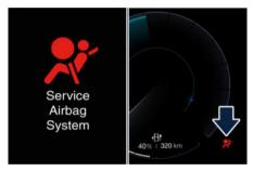
The air bag warning light monitors the internal circuits and interconnecting wiring associated with air bag system electrical components.
