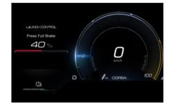
With brake pedal pressed full with left foot, fully press the accelerator pedal (with right foot) as indicated in the message on the instrument cluster.
