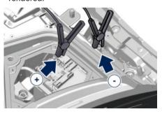
Start the booster battery and then start the electric motors in the vehicle with the discharged battery. Wait a few seconds after connecting the cables, before starting the booster.
