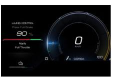
Release brake pedal. The launch of the vehicle starts with ESC that manages the maximum performance and electric motors torque calibrated to maximize performance.
