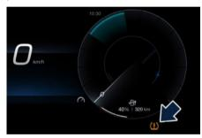
The vehicle may need to be driven for up to 20 minutes above 24 km/h (15 mph) in order for the TPMS to acquire and process the updated setting.
