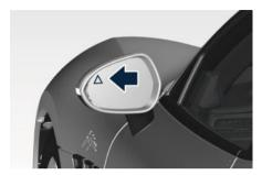
The external of the rear-view mirror support is equipped with LEDs, lighting up when the turn signals and vehicle entry/exit lights are activated.
