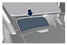
The Wireless Charger allows you to recharge your mobile phone (if it support this technology) without have to connect it to the charging port through a cable. The Wireless Charger system is designed to wirelessly charge mobile phones (maximum power available 15 W) compatible with the Qi ® standard. The system is activated in automatic mode when the mobile phone is placed in its compartment.
