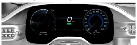
The layout of the instrument cluster consists of three active sectors. In the lateral ones **A** are only displayed the hard telltales, the central sector is configured with specific screen, depending on the drive mode selector position (see "Drive Mode" in section "Driving and Driver Assistance Systems").
