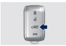
The so button on key fob does not only allow user to completely open the power boot lid, but also to invert its movement by pressing twice the button again. The power boot lid opening can be also operated from inside the vehicle pressing the button on front dome console.
