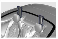
In addition to being ejected in the case of rollovers around the vehicle longitudinal axis (as shown in the figure) the active roll bars activate as a precautionary measure in the event of sufficiently severe side and rear collisions, and in all cases where the battery might be disconnected. They do not activate in the event of spinning.
