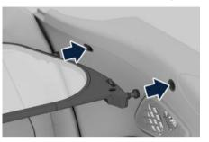
Holding the horizontal element of the Windstop only by the frame, lower the center section until you feel the parts engage.
