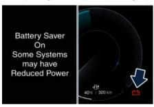
The vehicle contains advanced electronic systems, such as, for example, the alarm system and various electronic control modules, which consume power even when the ignition device is in **STOP** position and the vehicle is not being used.
