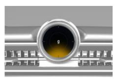
Filling of the halo is related to the real time acceleration value and it fills from the centre to the edge in the direction of the acceleration.
