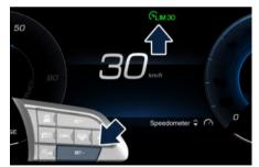
Pushing the button (SET +) or (SET -) once, or long pressing it will enable to increase or decrease the set speed by one unit (1 km/h or 1 mph).
