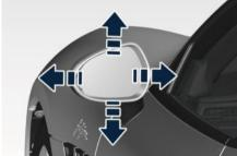
To adjust a rear view mirror, rotate the inner ring on **L** (left) or **R** (right) position to select the mirror that you want to adjust. A dot LED on it will illuminate indicating which rear view mirror is activated and can be adjusted. Press the mirror joystick switch to the direction of the desired movement. For optimal vision orientate the outside(s) mirror(s) in order to frame the adjacent lane and get a partial overlap with the
