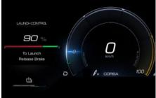
During the acceleration phase the "Launch Control" symbol appears at the left of the digital speedometer in the instrument cluster display.
