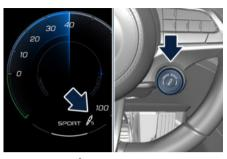
Pushing the  $\beta$  button, the telltale on the instrument cluster will be switched off.
