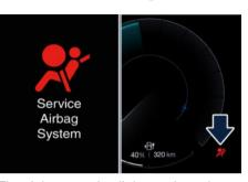
The air bag warning light monitors the internal circuits and interconnecting wiring associated with air bag system electrical components.
