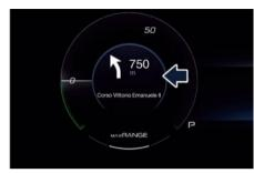
While getting closer to a turn, the sections referred to the distance already travelled will switch off while the ones. referred to the distance vet to be travelled will remain on.
