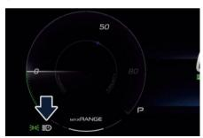
Once the high beams are physically on, the blue indicator on the left side of the cluster display comes on.
