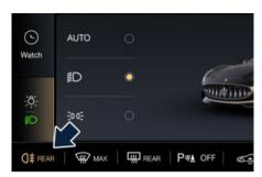
The rear fog light switches on only when the low beam lights are switched on. The light can be switched off by pressing the icon again or by switching off the low beam lights.
