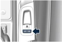
There is a single window control on the passenger door trim panel, which operate the corresponding window. The window controls will operate only when the ignition device is **ON** position.
