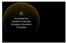
• The bulkhead in the boot (cargo spacer) is not positioned correctly.
