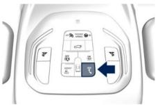
The manual SOS Call is always available, up to 10 minutes after Key OFF. In case of a software installation process is ongoing, the manual SOS Call is not available. When the connection between the vehicle and a safety operator is made, your vehicle will automatically transmit location and vehicle information to the service operator.
