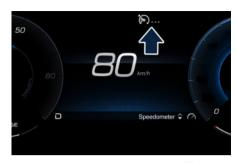
To turn the system off, push the NON/OFF button a second time. The Nowhite light will turn off.
