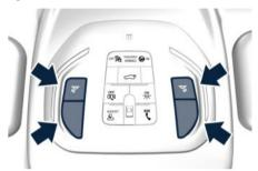
Both the lateral lights automatically turns on when one of the doors is opened and turns off when the door is locked and the ignition device is in **ON** position and if the greeting lights are active on the MIA screen (see paragraph "Functions of Controls Menu on MIA" in this section). The light may be switched on manually by pressing both buttons.
