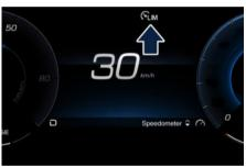
To disengage the system, push the same button a second time. The right will turn off and a new message pops up for 5 seconds, then the display returns to the previous setting.
