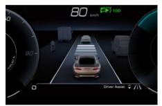
If another information covering ADAS visualization in the main area (textual pop ups, NAVI information, phone call, etc...) are displayed, the ACC time gap symbol shall be displayed in the top right corner for the time the ADAS in the main area is covered (see detail in picture). If system does not detect the presence of any vehicles ahead, only the bars
