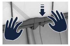
On the right-hand side of the horizontal element of the Windstop, move the fixing lever in the indicated direction.
