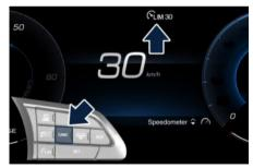
Pressing the brake pedal the SL function remains engaged, while the CC function, if it was active will be temporarily deactivated.
