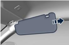
By lowering the sun visor you can access the courtesy mirror and, by opening the mirror protective cover, a LED light will
