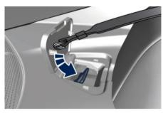
Tighten upper strap until you reach the tension level recommended by the restraint system manufacturer.
