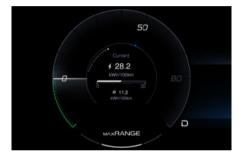
When speed is equal to 0 km/h or when the accelerator is not pressed or if the signal is not available, the gauge is empty and the instantaneous value is represented as dashes "--.-". Exceeding the maximum scale limit, the instantaneous numerical value shall be at least the upper limit of the scale.
