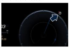
Every time a lap/sector time is taken the relative time gap is shown in overlay on the Smart Clock. Gap value is calculated comparing the time taken when a sector/lap is completed with the sector/lap of the best lap time of the session. Gap is not shown during first lap. Gap information is coloured in green when the time is lower/better, in red when is higher/worst.
