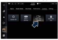
When displayed, dynamic grid lines (if the function is set to MIA through the "Settings" menu of the "Vehicle" page) will illustrate the width of the vehicle to assist with parking or aligning to a hitch/receiver. The dynamic grid lines will show separate zones in different colour that will help indicate the distance to the rear of the vehicle.
