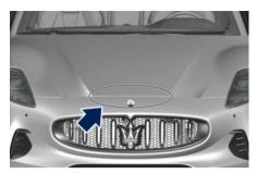
Slightly lift the hood and push the safety catch as indicated by the arrow.
