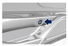
Alternatively, to release a front door from inside, pull the manual door emergency handle located under the latch door button.
