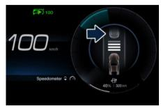
To increase or decrease the number of bars, corresponding to the time gap from vehicle ahead, press and release the related setting "pulse activation" button.
