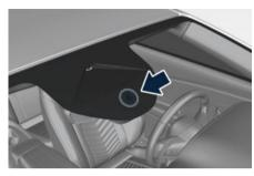
The sensor has an adjustment range which varies progressively from wiper still (no stroke) when the windshield is dry, to wiper at 2nd continuous speed (fast continuous operation) with intense rain.
