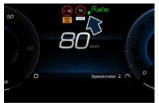
To accept the proposed speed and consequently adjust the speed set by the Speed Limiter, push the RES button. If ISA is set in "Manual" mode on the MIA screen, RES button confirm the suggested speed. If ISA is set in "automatic" mode on the MIA screen, the system will adapt automatically the speed, the driver can push RES within 5 seconds to reject the new speed. If the driver accepts the value suggested by the ISA or if the speed set using the
