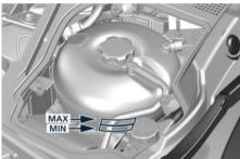
When additional refrigerant (antifreeze) is needed to maintain the proper level, contact the **Service Network** to have the reservoir refilled.
