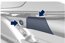
Once unlatched, the door is opened partially and then, with a slight push with the internal handle, automatically rotates outwards
