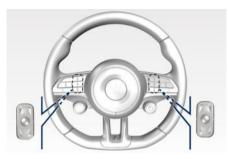
Press any button to display information on the radio station or track being listened to inside a pop up for 2 seconds on instrument cluster.
