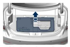
pull the release cord to manually unlock the actuator of the charging port;
