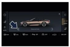
• Put the finger on each part of the display and make a swipe and hold gestures (slide/swipe from right to left) for the entire closing cycle.
