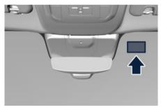
To apply the TAG (telepass), comply with the positioning dimensions compared to the upper edge of the windscreen and the centre line of the internal rearwiew mirror, shown in picture.
