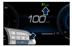
Release the accelerator and the vehicle will operate at the selected speed.
