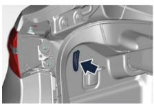
Remove the right side plug inside the boot to reach the small cables to unlock the soft top cover locks.
