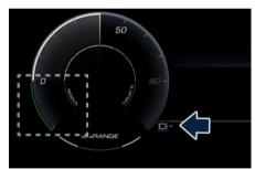
Telltales are shown near the gearshift indicator in order to advise the user that the function is activated and its level. The gearshift and powermeter regen cluster area display the status of the e-Coasting system (D-- / D- / D / D+). The D-- corresponds to the max recovery.
