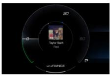
The screen will be updated at the start of each new song; available information will depend on the song. Buttons on the rear of the steering wheel are effective on Media. If the selected widget is different from the Media/Radio widget, no feedback is provided when the user changes track / station.
