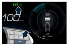
Remove foot from accelerator pedal and vehicle will continue at set speed.
