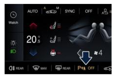
The soft-key will be on in an amber colour when the entire Park Assist system is temporally disabled or not activated in the setting list. The soft-key will turn white when the system is enabled again.
