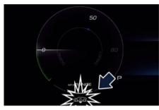
If the vehicle overcome the 50 km/h (31 mph) maximum speed, the lifter lowers automatically the vehicle to the normal height and a pop-up with the lowering description is shown on the instrument cluster. If the user try to activate the lifter, a pop-up will display in order to warn him that the lifter is not available at this speed.
