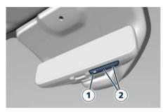
To adjust the display brightness, press the button to select the icon. Press left adjustment button to darken or press the right adjustment button to brighten.
