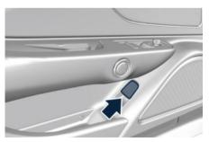
The door latch will then release, allowing the door to be partially opened before it automatically swings outwards.
