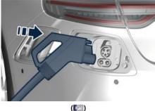
If the first and last LEDs on the vehicle charging port flash red, start charging from the column according to the starting procedure recommended by its operator (e.g. press the START button). If the LEDs on the vehicle charging port do not light, disconnect the adapter and reconnect it, then wait for the two LEDs to flash red and start charging from the column:
