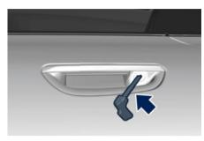
Rotate the emergency key in order to align the reference marks present on the cap and the handle body.
