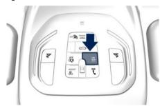
The lighting of all the compartment lights when opening the doors can also be inhibited by pushing the indicated button.
