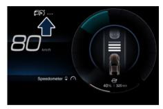
Push the ON/OFF button a second time and release to turn the system off. A pop up message is displayed for 2 seconds to indicate that ACC was disabled.
