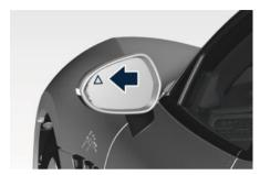
The BSA detection zone shown in figure covers approximately one lane on both sides of the vehicle. The blind spot area extends from immediately behind the exterior rear-view mirrors up to behind the rear bumper.
