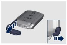
To reassemble the key fob push the emergency key back into the key body till the release button returns in his original location.
