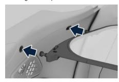
Perform the same operation to engage the opposite pins on the left side of the horizontal element of the Windstop.
