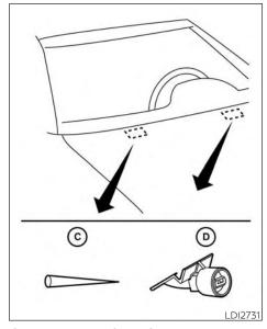
If you wax the surface of the hood, be careful not to let wax get into the washer nozzle O. This may cause clogging or improper windshield-washer operation. If wax gets into the nozzle, remove it with a needle or small pin O.
