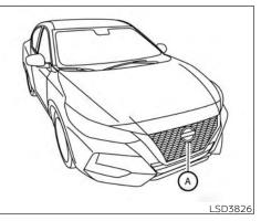
The I-FCW system uses a radar sensor A located on the front of the vehicle to measure the distance to the vehicle ahead in the same lane.
