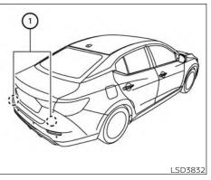
The RCTA system uses radar sensors () installed on both sides near the rear bumper to detect an approaching vehicle.
