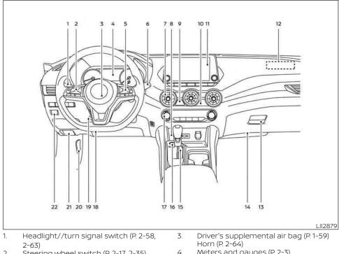
Steering wheel switch (P. 2-17, 2-35) 2. Audio controls (P. 4-63)
