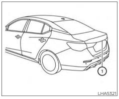
To display the rear view, the RearView Monitor system uses a camera located just above the vehicle's license plate  $\bigcirc$ .
