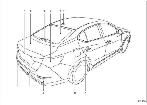
8. Fuel-filler door (P. 3-22) Fuel-filler cap (P. 3-22) Fuel recommendation (P. 10-4)
