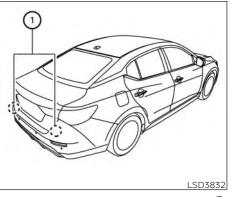
The BSW system uses radar sensors  $\bigcirc$  installed near the rear bumper to detect other vehicles in an adjacent lane.
