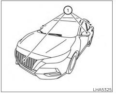
If dirt, rain or snow accumulates on any of the cameras ①, the Intelligent Around View<sup>®</sup> Monitor may not display objects clearly. Clean the camera by wiping with a cloth dampened with a diluted mild cleaning agent and then wiping with a dry cloth.
