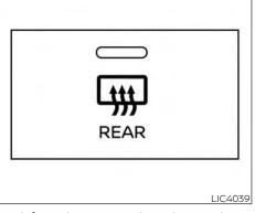
To defrost the rear window glass and outside mirrors (if so equipped), start the engine and push the rear window defroster switch on. The rear window defroster indicator light on the switch comes on. Push the switch again to turn the defroster off.
