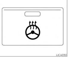
The heated steering wheel system is designed to operate only when the surface temperature of the steering wheel is below  $68^{\circ}F$  (20°C).
