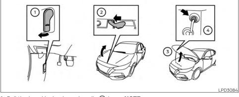
1. Pull the hood lock release handle ① located on the lower door pillar until the hood springs up slightly.
