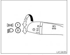
Type A (if so equipped) HEADLIGHT CONTROL SWITCH
