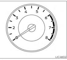
**7 inch (18 cm) Type B (if so equipped)** Do not rev the engine into the red zone ①.
