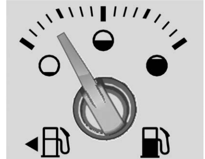
Midlevel Metric Fuel Gauge Shown, Base Level and Uplevel Fuel Gauge Similar
