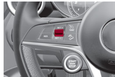
SET Switch Location
