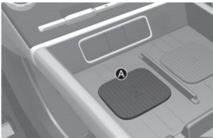
[A] Vehicle authentication pad (Wireless charging pad)
