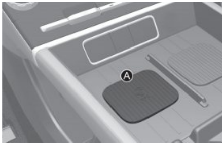
[A] Vehicle authentication pad (wireless charging pad)
