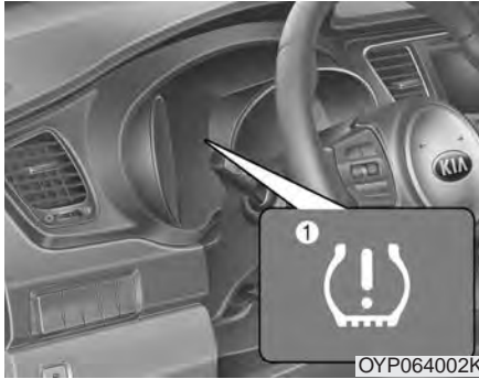
(1) Low tire pressure telltale / TPMS malfunction indicator
