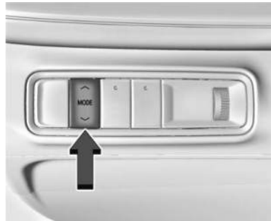
Driver Mode Control Switch
