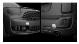
Threaded holes for the tow fitting are located in the front and rear of the vehicle on the right side with respect to the direction of travel.
