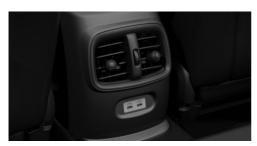
One USB dual charge socket is located in the rear center console.
