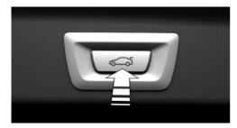
Press the button on the inside of the tail-gate.
