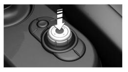
Tilt in four directions to switch between displays, for example.
