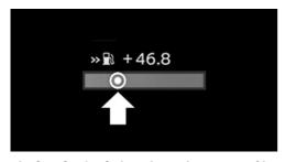
The bar display below the tachometer is filled in green and the mark appears at the zero point. The tachometer indicates idle speed.
