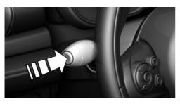
Press the button on the turn signal lever. Information is displayed in the instrument cluster.
