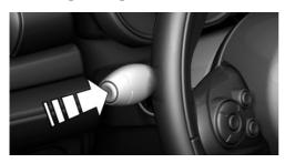
Press and hold the button on the turn signal lever.
