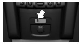
The USB port is located in the front of the center console.
