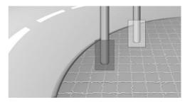
Depending on the vehicle equipment, obstacle markings can be faded into the image of the rearview camera.
