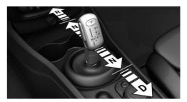
The selector lever positions R, N, and D are selected by tapping the selector lever for-
