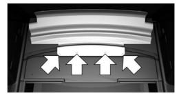
Fold down the MINI Picnic Bench toward the rear. The MINI Picnic Bench is fastened with magnets.
