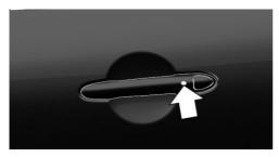
On the driver's or front passenger's outer door handle, press the button.
