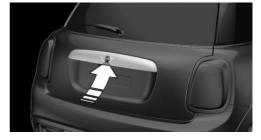
Without Comfort Access: unlock vehicle. With Comfort Access: unlock the vehicle or have the vehicle key with you. Press button next on tailgate.
