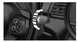
Turn the thumbwheel on the wiper lever.
