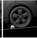
If you need to change a wheel on a slight downhill grade, place chocks and other suitable objects, for instance a rock, under the wheels of both the front and rear axles against the rolling direction.
