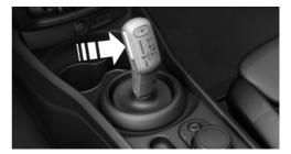
2. With the driver's safety belt fastened, briefly push the selector lever in the desired direction, past a resistance point, if needed. The selector lever automati-
