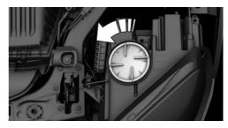
3. Turn the bulb holder counterclockwise, arrow 1, and remove, arrow 2.
