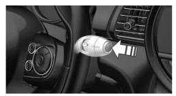
Press the button on the wiper lever.
