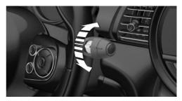
Turn the thumbwheel on the wiper lever.
